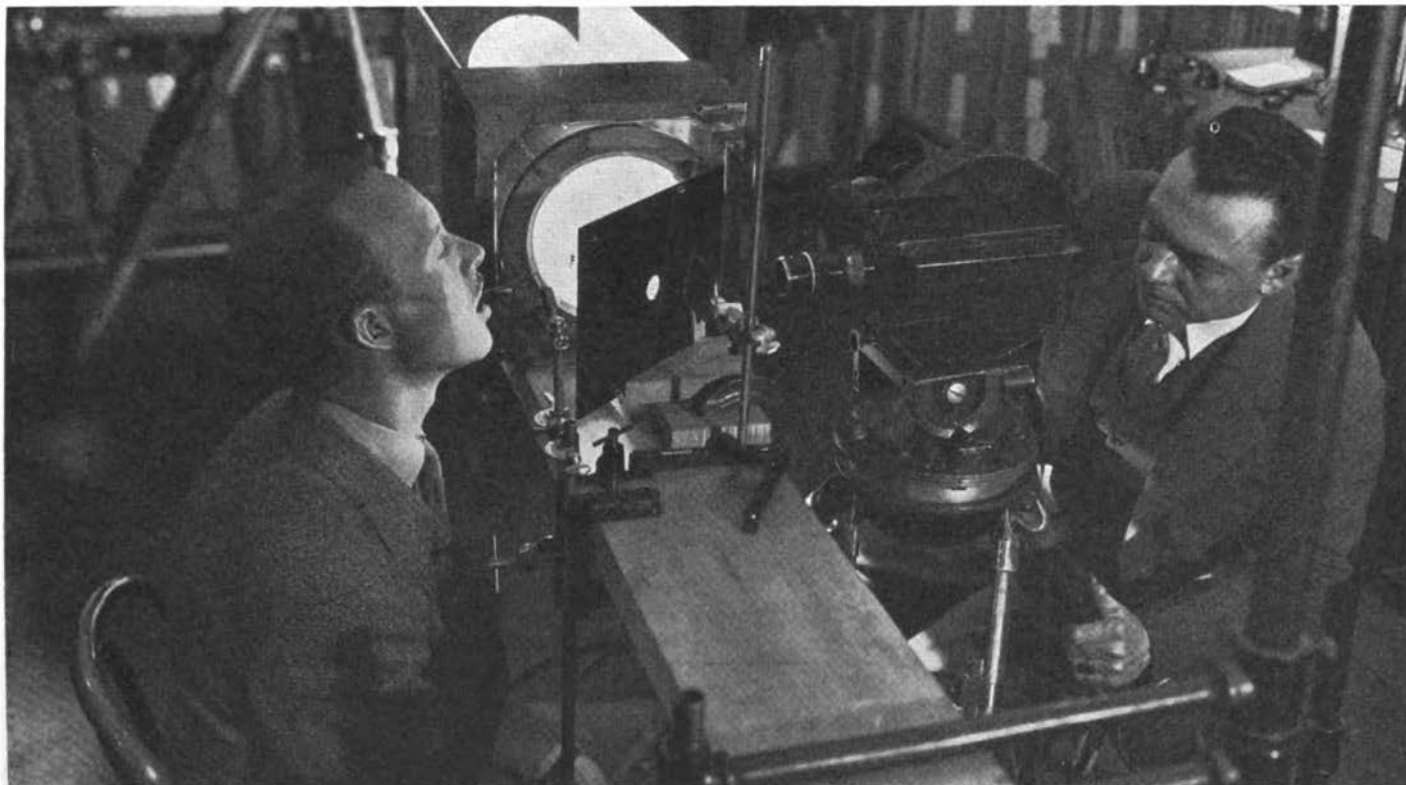
FIGURE 18.—High-Speed Motion Pictures of the Human Vocal Cords, Bell Telephone Laboratories, New York, New York 274235—41—8
