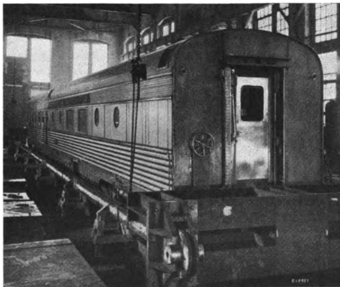
FIGURE 99.—"Squeeze" Test Machine for Subjecting Passenger Cars to Compression Load of 900,000 pounds, Pennsylvania Railroad Research Laboratories, Altoona, Pennsylvania
