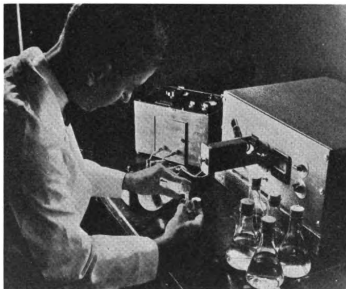
FIGURE 81.—Photoelectric Colorimeter for Measuring Amount of Vitamin A in Foods, Purina Mills, St. Louis, Missouri
