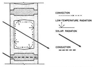
Fig. 1.21—Heat exchanges within a glass block panel. 24
