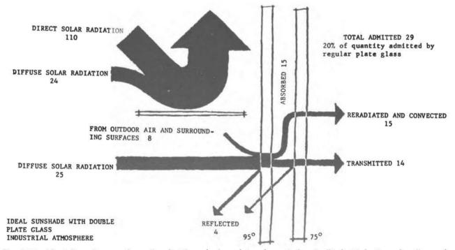
Fig. 3.11—Heat flow diagram for a "perfect" sunshade—plate glass window in "industrial atmosphere"—peak load for worst orientation.
