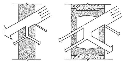
183 BTU/HR-SQ FT 91 BTU/HR-SQ FT Fig. 1.22—Comparison between regular window glass and a glass block panel.
