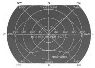
Fig. 3.8—Maximum solar radiation on vertical walls, August I, No.v York, N. Y.
