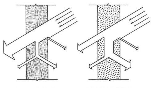
183 BTU/HR-SQ FT I26 BTU/HR-SQ FT Fig. 1.17—Comparison between regular window glass and heat-absorbing glass.
