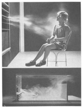
Fig. 1.30—Direct drafts are essential to summer comfort in hot, humid weather.
