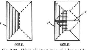
Fig. 2.29—Effect of introduction of a horizontal member.
