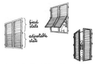
Fig. 2.8—Traditional shutters. Closed (left) they keep out rain and sun, let air circulate. For more air and some view, the lower half opens awning-wise (center). Swung half open (right) the two leaves act as vertical sun shades.
