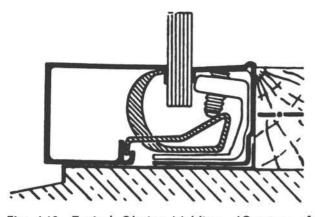
Fig. 4.12—Typical Glazing Molding. (Courtesy of Kawneer Co.)
