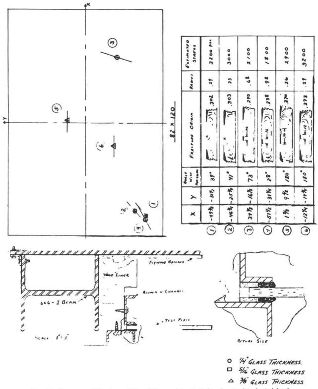
Fig. 2.2—Summary of fracture origins of large plates tested under simulated wind loads.
