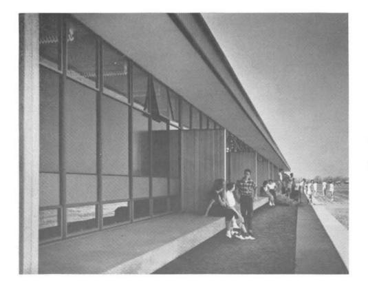
Fig. 4.32—Combination of clear and glare-reducing glass with roof overhang, Norman High School, Norman, Okla.
