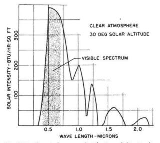
Fig. 1.12—Spectral energy distribution of direct solar radiation at sea level.
