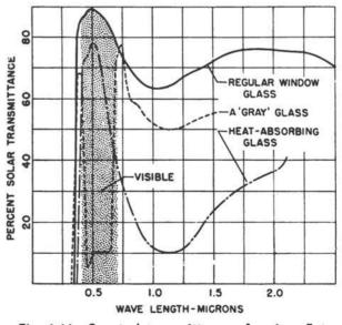
Fig. 1.16—Spectral transmittance of various flat glasses.
