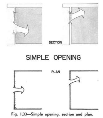
In Figs. 1.33, 1.34, 1.35, typical air patterns are shown in section (above) and plan (below), assuming a wind perpendicular to the plane of the window wall.
