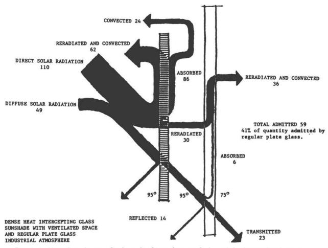
Fig. 3.12—Heat flow diagram for heat-absorbing glass, sunshade and freely ventilated air space.
