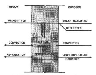
Fig. 1.15—Instantaneous heat balance for any fenestration.
