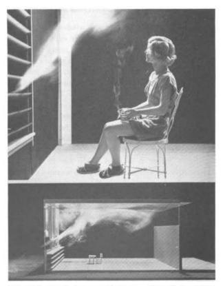
Fig. 1.29—Draft-free ventilation: a "must" in winter, a mistake in summer.
