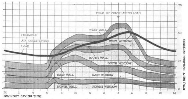
Fig. 3.10—Total instantaneous heat gain due to walls and windows for a square tower with 25% window area, oriented with Manhattan street pattern, August 1.
