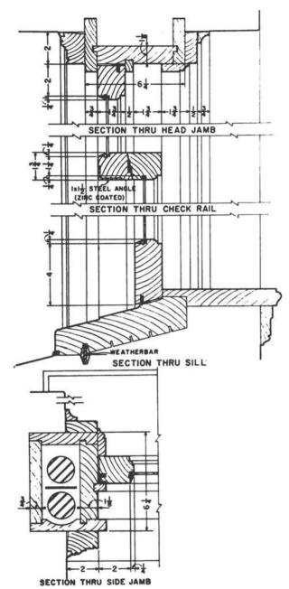
Fig. 2.14—Typical double-hung window and frame for institutional type building.
