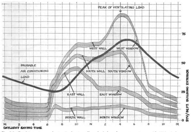
Fig. 3.9—Total instantaneous heat gain due to walls and windows for a square tower with 50% window area, oriented with Manhattan street pattern, August 1.
