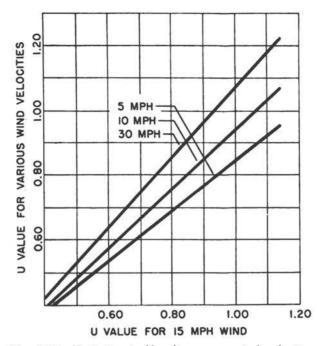
Fig. 1.23—Variation in U value versus wind velocity.
