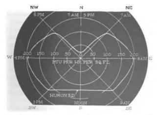
Fig. 3.7—Maximum solar radiation on vertical walls, August I, Huron, S. D.
