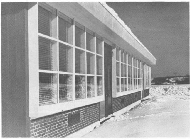
Fig. 4.23—Use of double glazing at Millinocket School.
