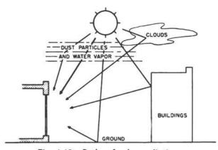
Fig. 1.13—Paths of solar radiation.
