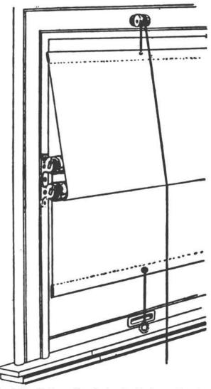
Fig. 3.16—Spring roller shades double hung at center of window.
