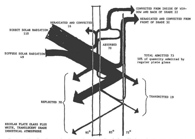
Fig. 3.13—Heat flow diagram for white finish inside window shade or blind completely covering window.
