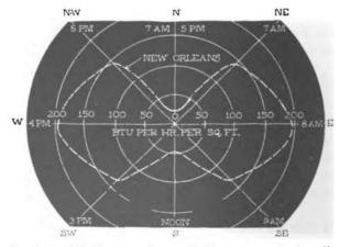
Fig. 3.6—Maximum solar radiation on vertical walls, August I, New Orleans, La.
