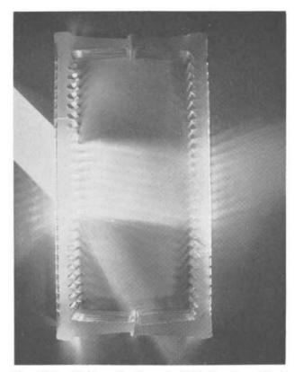
Fig. 2.18—Light path through light-directing block section.
