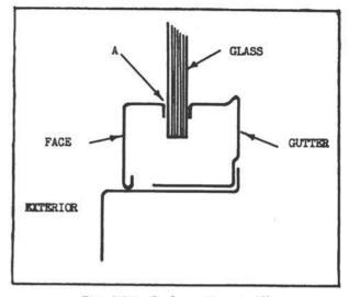
Fig. 2.27—Sash section at sill.
