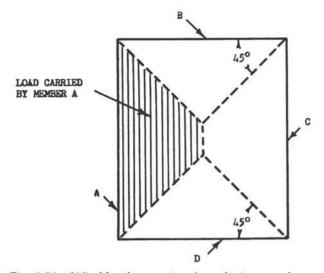
Fig. 2.28—Wind load transmitted to glazing members.
