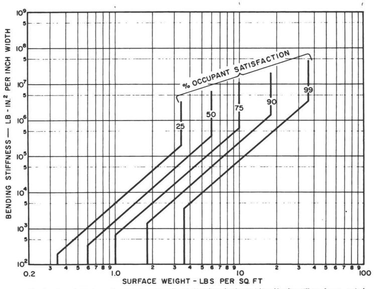
Fig. 1 - Approximate degree of speech privacy for walls with the indicated surface weight and bending stiffness, for one, typical, between-office situation.
