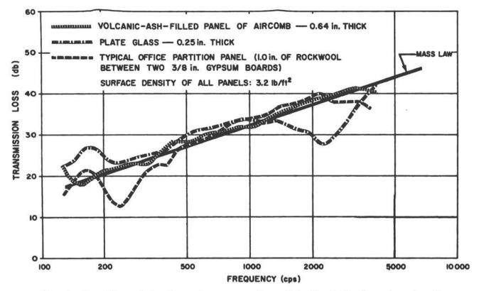
Fig. 1 - Sound Transmission Loss vs Frequency - Comparison of acoustical panels made with honeycomb core with two conventional panels of equal weight.
