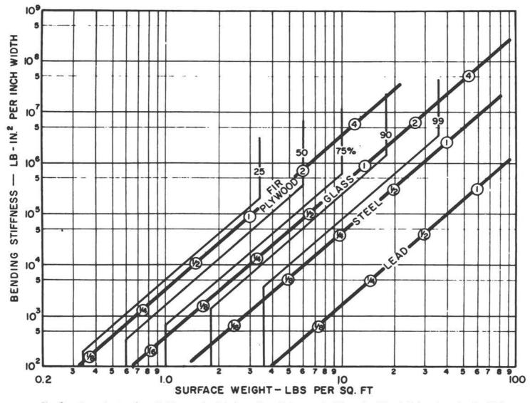
Fig. 2 - Approximate values of stiffness and weight for various thicknesses of solid panels. The circled numbers give the thickness in inches.
