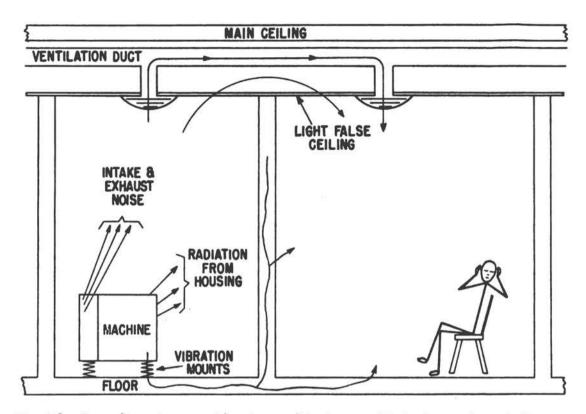
Figure 1 - Two adjacent rooms with noisy machine in one. Typical acoustic and vibration paths are indicated.
