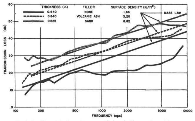
Fig. 2 - Sound Transmission Loss vs Frequency - Filled panels of honeycomb material: same thickness, different fillers.
