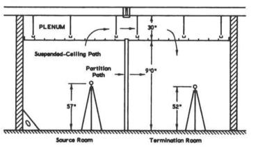
Figure 1 Schematic Section Through Two-Room Suspended-Ceiling Facility
