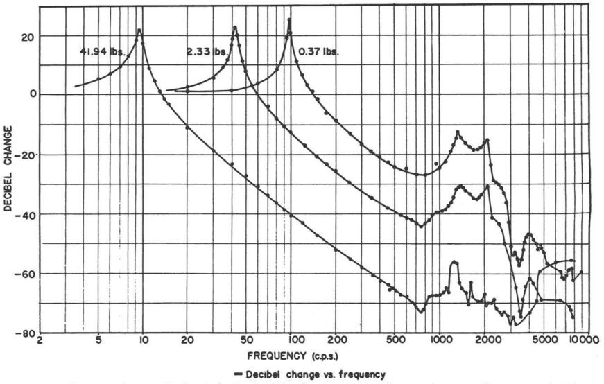
Figure 4 – Measured attenuation of a simple vibration isolated system consisting of a mass, shear type rubber mount, and rigid foundation. (After Muster)
