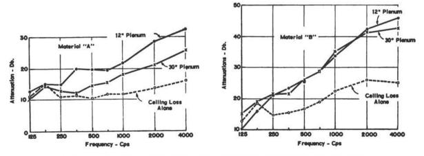
Fig. 7 - Two-Room Attenuation Spectra Compared to Transmission Loss
