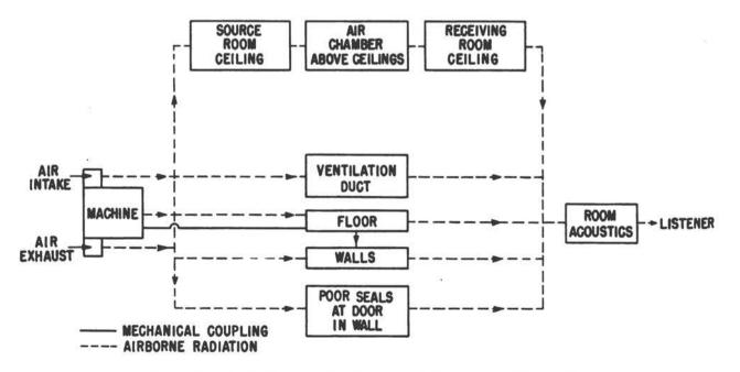
Figure 2 - Block diagram of noise transmission paths of Figure 1.
