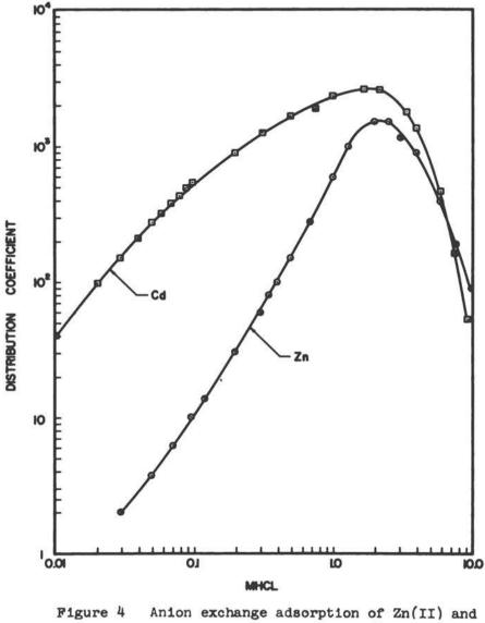
Figure 4 Anion exchange adsorption of Zn(II) and Cd(II). (Taken from Kraus and Nelson 83 )
