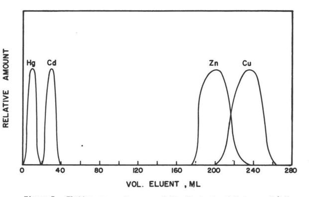
Figure 3 Elution curves for some of the divalent metal ions. 0.4 M HCl used as eluent; ion exchange resin, Dowex 50x4, 200-400 mesh. (Taken from UCRL 2531<sup>72a</sup>.)
