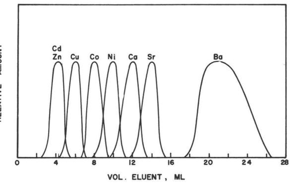
Figure 2 Elution curves for some of the divalent metal ions; 3.1 M HCl used as eluent; ion exchange resin, Dowex 50x4, 200-400 mesh. (Taken from UCRL 2531<sup>72a</sup>.)
