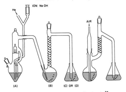
Fig. 3. Apparatus for separation and purification of  $N^{13}H_{3}$ .
