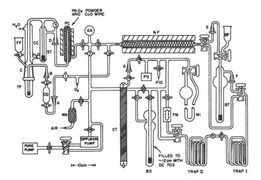
Fig. 2. Vacuum line for separating and purifying  $C^{11}$
