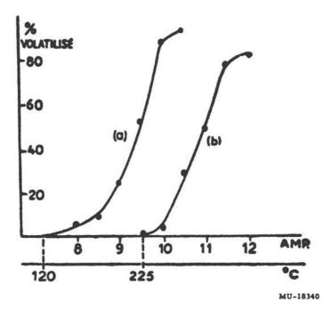
Fig. 3. Volatilization of francium from an electrically heated platinum filament. Francium evaporated on the filament as a chloride solution. (a) In vacuum (b) in air.
