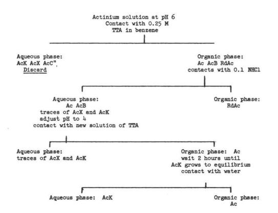
This method does not work at all well if the actinium source contains a great quantity of rare earth elements because the solubility of the TTA complexes in benzene is rather limited. There are some other disadvantages. For example, it takes several minutes of stirring before the complex is formed and extracted. Also the extraction coefficients lie in the range of 20 to 100 and are not so large that a clean separation can be made in a single extraction.
