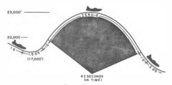
Figure 35. F-94C Zero-G "SAM" Flight Parabola: The maneuver is started at an altitude of about 18,000 feet, reaches about 23,000 feet at the top of the parabola, and yields about 40 seconds of virtual weightlessness.
