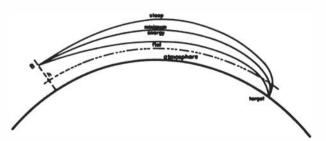
Figure 50. Schematic Representation of Missile Trajectories with Different Launching Angles
