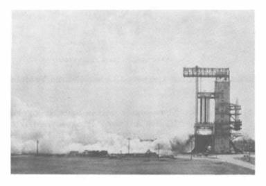
Figure 65. SATURN Booster During Static Firing
