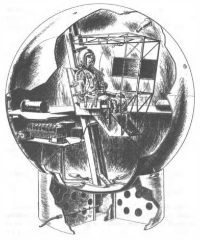
Figure 75. Martin Reaction Control Simulator General Arrangement of Basic Unit
