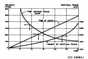
Figure 20. Sled Velocity Parameters
