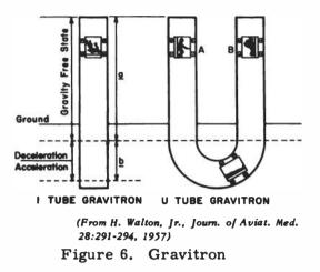
3. Figure 7 shows typical velocity and gravity cycles in an I-gravitron. Zero-G states are alternating with states of increased acceleration. The vertical tube has a height of 350 m (1,148 feet). This would allow a zero-G state of about 14 seconds, and deceleration-acceleration at 4 g for 4.66 seconds.
