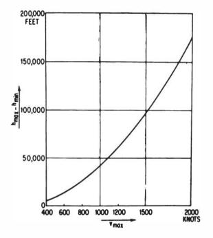
Figure 26. Height of the parabolic arc vs maximal speed, for a minimal speed of 200 knots.
