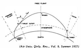
Figure 49. Trajectory of an ICBM
