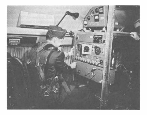
Figure 31b. Psychomotor Performance Test During Zero-G in the C-131B.
