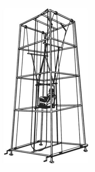
Figure 5. Subgravity Tower
