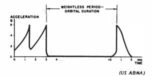
Figure 17. Typical Acceleration Pattern Two-Stage Booster
