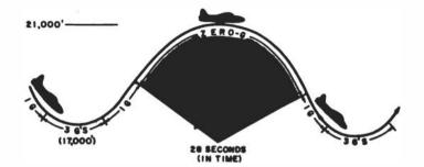
Figure 33. T-33 Zero-G SAM Flight Parabola: The maneuver starts at an altitude of about 18,000 feet, reaches almost 21,000 feet at the top of the parabola, and yields about 28 seconds of virtual weightlessness.
