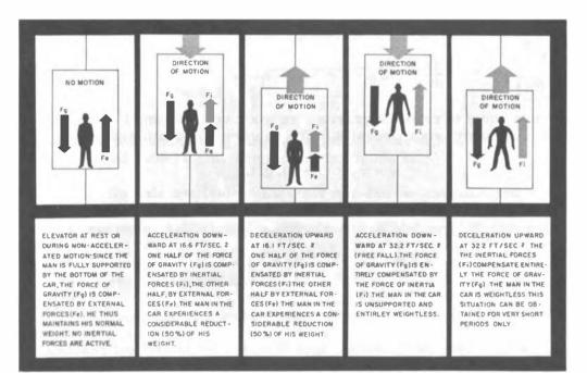
Figure 4a. Sub-gravity and Zero-G in Elevators
