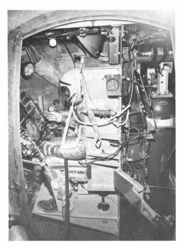
Figure 4. Johnsville centrifuge: centrifuge on which Astronauts were given experience with launch and reentry acceleration profiles. Note that provisions have been made for use of full-pressure suit and for decompression of the gondola. Astronauts are also provided with simulation of Mercury instrument panel and hand controller.
