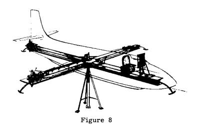
of gravity. To power the rockets mounted at the extremes of the I-beams, hydrogen-peroxide fuel is metered through a valve and is activated by a silver-screen catalyst. The Iron Cross was devised primarily to check operational characteristics of the rockets and control-system hardware, and was found to be inferior to the analog as a training device.
