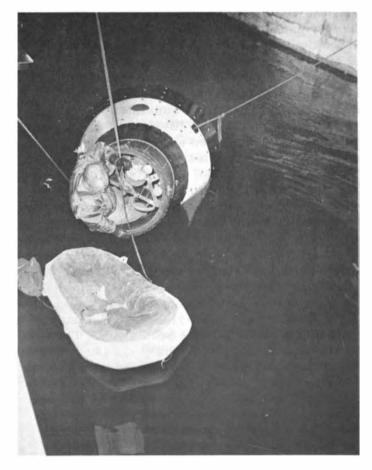
Figure 8. Environmental control system simulator: a device consisting of a mock capsule with a flighttype environmental control system which can be placed within a decompression chamber to simulate the operation of the environmental control system during the Mercury flight.
