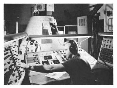
Figure 6. Mercury procedures simulator: a fixedbase trainer which permits practice in management of Mercury systems and attitude control. From instructor's console in foreground, faults can be inserted into any of the Mercury indicators. Astronaut's corrective action is signaled by lights on panel.
