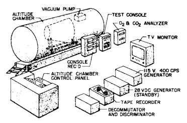
Figure 7. Environmental control system simulator: a device consisting of a mock capsule with a flighttype environmental control system which can be placed within a decompression chamber to simulate the operation of the environmental control system during the Mercury flight.
