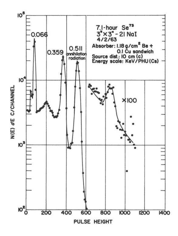
FIGURE 2, Gamma-ray spectrum of 7.1-hour Se<sup>73</sup>.
