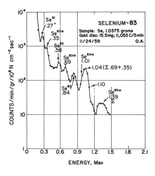
FIGURE 6, Gamma-ray spectrum of Se<sup>83</sup>.
