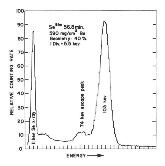
FIGURE 5, Gamma-ray spectrum of 56.8 min. Se<sup>81 m</sup>,
