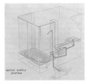
Fig. 4. Tub and walls to be added to lavatory-water closet component.
