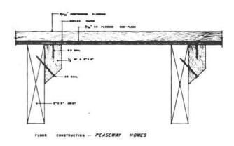
Fig. 4. Floor construction
