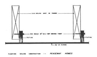
Fig. 5. Floating ceiling construction
