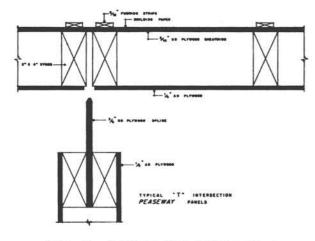
Fig. 3. Typical "T" intersection
