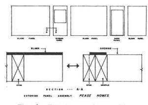
Fig. 6. Exterior panel assembly
