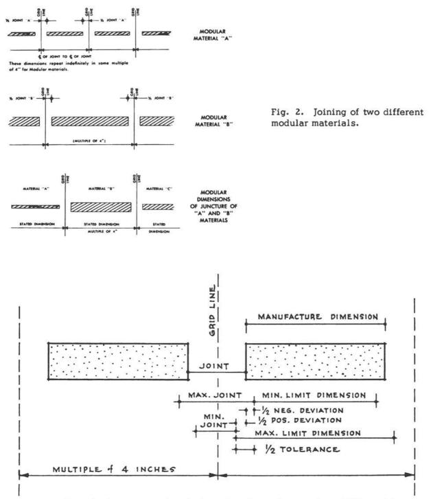
Fig. 3. Note drafting convention designating dimensions to the grid line with an arrowhead and to the off-grid point with a dot.
