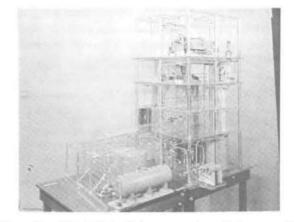
Fig. 7. Completed true-scale piping model with all phases such as electrical and mechanical shown.
