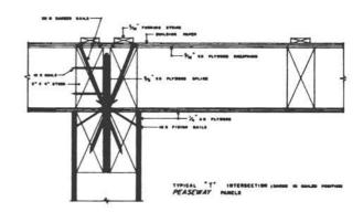
Fig. 2. "T" intersection nailed in place
