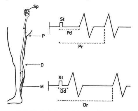
Fig. 1.--Method Used for Measuring Various Temporal Components of the Human Monosynaptic Spinal Reflex
