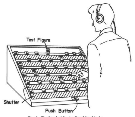
Fig. 3.--The Standard Sorting Board Used in the Speed of Identification Task. Note:--Test figure appears once in each row. As soon as shutter opens, S locates test figures, turns them over, and pushes button to signify completion of a trial.
