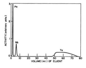
FIGURE 4 SEPARATION OF PROTACTINIUM (文), NIOBIUM(文) AND TANTALUM(文) BY ANION EXCHANGE: 12.5 cm. DOWEX -I COLUMN, 0.0226 sq. cm. CROSS-SECTION, 0.3ml. minute<sup>-1</sup> FLOW RATE, ELUENT 9 M HCI-0.05 M HF
