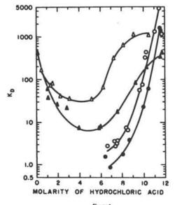
Figure 6 Dependence of the distribution coefficient at 250 on the hydrochioric acid concentration:  $\triangle$ , niobium;  $\triangle$ , tantaium;  $\bigcirc$ , zirconium;  $\oplus$ , hafnium.
