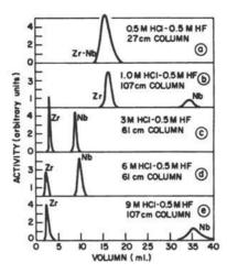
FIGURE 3 SEPARATION OF Zr AND Nb WITH DOWEX-I ANION EXCHANGE COLUMNS: AVERAGE FLOW RATE co.0.3 mL/sq.cm/minute; CROSS-SECTION OF COLUMN:0.0226 sq.cm
