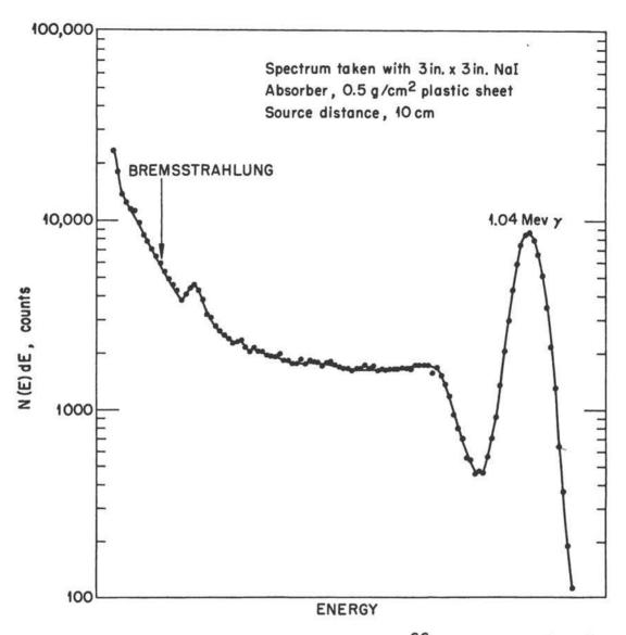
Fig. 6. Gamma-ray spectrum of Cu<sup>66</sup>, half-life = 5.1 min.
