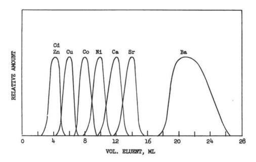
Figure 1. Elution curves for some of the divalent metal ions; 3.1 <u>M</u> HCl used as eluent; ion exchange resin, Dowex 50, 200-400 mesh. (Taken from UCRL-2531.<sup>(82)</sup>)
