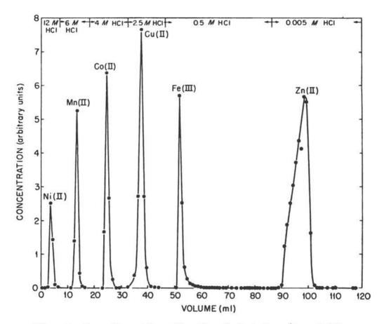
Figure 3. Separation of Transition Elements Mn to Zn. (Dowex-1 Column; 26 cm x 0.29 cm., flowrate = 0.5 cm/min.). Taken from Kraus, K. A. and Moore, G. E., <u>J. Am. Chem. Soc.</u>, <u>75</u>, 1460 (1953).
