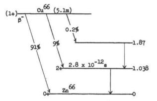
Figure 5. Decay Schemes of Copper-64 and Copper-66. Taken from Strominger, D., Hollander, J. M., and Seaborg, G. T., <u>Rev. Modern. Phys.</u> <u>30</u>, 585-903 (1958).
