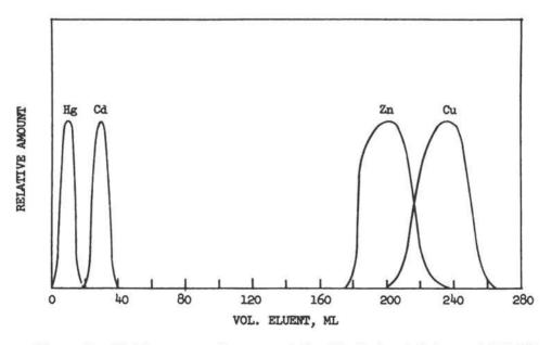
Figure 2. Elution curves for some of the divalent metal ions; 3.1 <u>M</u> HCl used as eluent; ion exchange resin, Dowex 50, 200-400 mesh. (Taken from UCRL-2531.<sup>(82)</sup>)
