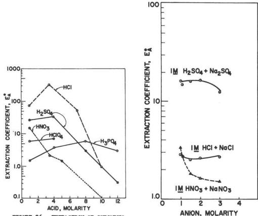
FIGURE 26. EXTRACTION OF CHROMIUM (VI) WITH TRI-N-OCTYLPHOSPHINE OXIDE EFFECT OF CONCENTRATION OF ACID. Chromium - 10.3 mg; TOPO -0.1 M in cyclohexane, 5 ml; Phase ratio - 1; and Extraction time -10 minutes.
