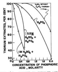
FIGURE 43. EFFECT OF SULFATE AND PHOSPHATE ON THE EXTRACTION OF THORIUM FROM NITRATE SOLUTIONS WITH TRI-N-OCTYLPHOSPHINE OXIDE. Thorium - 0.345 mg; TOPO - 0.1 M in cyclohexane, 5 ml; HNO<sub>3</sub> - 0.5 M; NaNO<sub>3</sub> - 4 M; and Phase ratio - 1.
