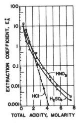
FIGURE 24. EXTRACTION OF BISMUTH FROM ACIDIC SOLUTIONS BY TRI-N-OCTYLPHOSPHINE OXIDE AS A FUNCTION OF TYPE AND CONCENTRATION OF ACID. Bismuth - 20 mg; HNO<sub>3</sub> - 0.5 M; TOPO - 0.1 M in cyclohexane, 5 ml; Phase ratio - 1; and Extraction time - 10 minutes.
