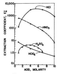
FIGURE 46. EXTRACTION OF URANIUM (VI) WITH TRI-N-OCTYLPHOSPHINE OXIDE AS A FUNCTION OF ACID CONCEN-TRATION. Uranium - 9 mg; TOPO -0.1 M in cyclohexane, 5 ml; Phase ratio - 1; and Extraction time -10 minutes.
