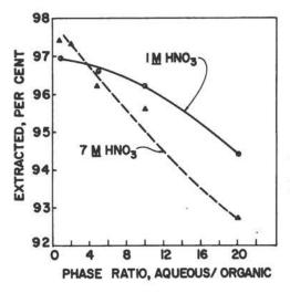
FIGURE 38. EXTRACTION OF CERIUM(IV) WITH TRI-N-OCTYLPHOSPHINE OXIDE AS A FUNCTION OF PHASE RATIO. Cerium - 21 mg; TOPO - 0.1 <u>M</u> in cyclohexane, 5 ml; and Extraction time - 10 minutes.
