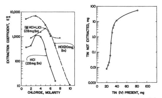
FIGURE 16. EXTRACTION OF TIN(IV) WITH TRI-N-OCTYLPHOSPHINE OXIDE AS A FUNCTION OF CHLORIDE CONCENTRATION. TOPO - 0.1  $\underline{M}$ in cyclohexane, 5 ml; Phase ratio - 1: Extraction time - 10 minutes.
