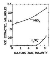
The solubility of the TOPO-acid adduct in the cyclohexane phase varies with the acid used. The perchloric acid adduct becomes immiscible in systems that contain 3 M HClO<sub>4</sub> or greater and forms an intermediate, third phase. A third phase is also produced when the concentration of sulfuric acid exceeds 8 M. Nitric and hydrochloric acids form adducts that are completely soluble in cyclohexane and represent the systems most favorable for the extraction of cationic substances.
