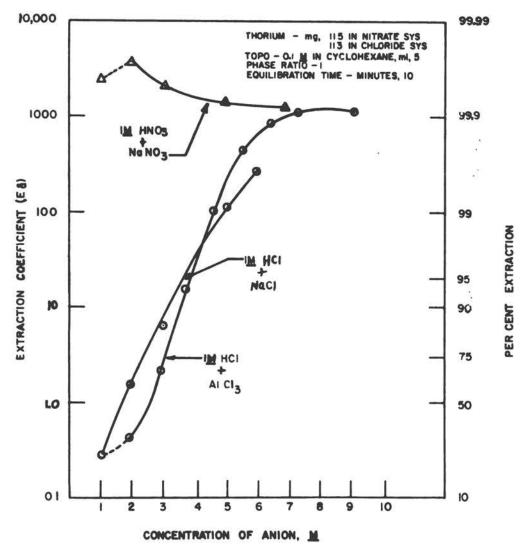
FIGURE 40. EFFECT OF CONCENTRATION OF CHLORIDE AND NITRATE ON THE EXTRACTION OF THORIUM WITH TRI-N-OCTYLPHOSPHINE OXIDE
