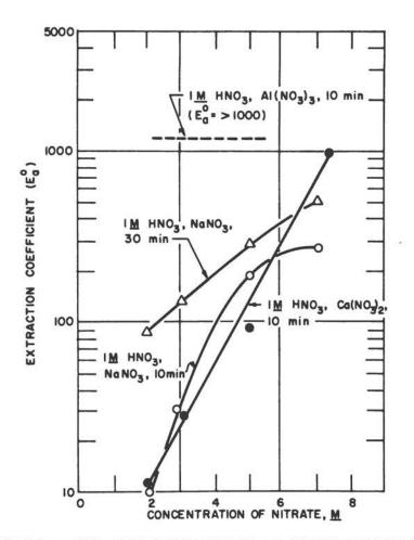
FIGURE 10. EXTRACTION OF ZIRCOVIUM BY 0.1 M TRI-N-OCTYLPHOSPHINE OXIDE AS A FUNCTION OF THE CONCENTRATION OF NITRATE SALTS OF UNI-, DI-, AND TRI-VALENT METALS. 2r - 9.35 mg; TOPO - 0.1 M in cyclohexane, 5 ml; and Phase ratio - 1.
