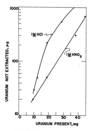
FIGURE 48. EXTRACTION OF URANIUM TTH TRI-M-OCTYLPHOSPHINE OXIDE. TOPO - 0.1 <u>M</u> in cyclohexane, 5 ml; Phase ratio - 1, and Equilibration time, 10 minutes.
