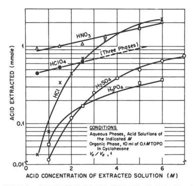
FIGURE 1. EXTRACTION OF MINERAL ACIDS FROM AQUEOUS SOLUTIONS WITH TRI-N-OCTYLPHOSPHINE OXIDE
