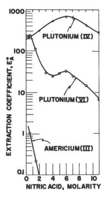
FIGURE 52. EXTRACTION OF PLUTONIUM FROM HC1 WITH TRI-N-OCTYLPHOSPHINE OXIDE. TOPO - 0.1 M in cyclohemane; Phase ratio - 1; and Extraction time - 10 minutes.
