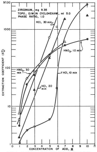
Figure 8. Effect of acid concentration and extraction time on the extraction of zirconium with 0.1  $\underline{M}$  TRI-N-OCTYLPHOSPHINE OXIDE
