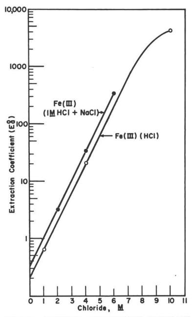
FIGURE 33. EXTRACTION OF IRON FROM CHLORIDE SOLUTIONS WITH TRI-N-OCTYLPHOSPHINE OXIDE. Fe -8 mg; TOPO -0.1 M in cyclohexane, 5 ml; Phase ratio -1; and Extraction time -10 minutes.
