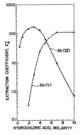
FIGURE 21. EXTRACTION OF ANTIMONY WITH TRI-N-OCTYLPHOSPHINE OXIDE AS A FUNCTION OF HYDROCHLORIC ACID CONCENTRATION. Antimony(III) -10 mg; Antimony(V) - 9 mg; TOPO -0.1 M in cyclohexane, 5 ml; Phase ratio - 1; and Extraction time -10 minutes.
