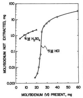
FIGURE 32. EXTRACTION OF MOLYBDE-NUM(VI) WITH TRI-N-OCTYLPHOSPHINE OXIDE AS A FUNCTION OF MOLYBDENUM CONCENTRATION. TOPO - 0.1 M in cyclohexane, 5 ml; Phase ratio - 1; and Extraction time - 10 minutes.
