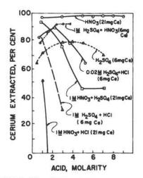
FIGURE 36. EXTRACTION OF CERIUM(IV) WITH TRI-N-OCTYLPHOSPHINE OXIDE AS A FUNCTION OF ACID CONCENTRATION. TOPO - 0.1 M in cyclohexane, 5 ml; Phase ratio - 1; and Extraction time - 5 minutes.
