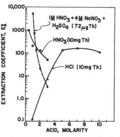
FIGURE 1.1. EXTRACTION OF THORIUM WITH TRI-N-OCTYLPHOSPHINE OXIDE RADIOTHORIUM-234 SYSTEMS. TOPO -0.1 M in cyclohexane, 5 ml; Phase ratio - 1; and Extraction time -15 minutes.
