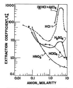
FIGURE 31. EXTRACTION OF MOLYBDE-NUM(VI) FROM ACIDIC SOLUTIONS WITH TRI-N-OCTYLPHOSPHINE OXIDE AS A FUNCTION OF ACID CONCENTRATION. Mo<sup>+6</sup> - 19.8 mg; TOPO - 0.1 M in cyclohexane, 5 ml; Phase ratio - 1; and Equilibration time - 10 minutes.
