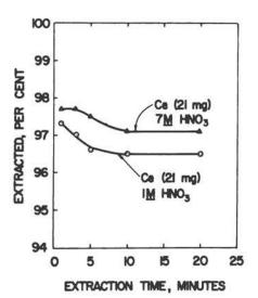
FIGURE 37. EXTRACTION OF CERIUM(IV) WITH TRI-N-OCTYLPHOSPHINE OXIDE AS A FUNCTION OF EXTRACTION TIME. TOPO - 0.1 <u>M</u> in cyclohexane, 5 ml; and Phase ratio - 1.
