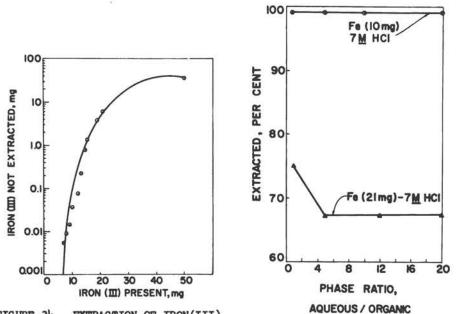
FIGURE 34. EXTRACTION OF IRON(III) WITH TRI-N-OCTYLPHOSPHINE OXIDE AS A FUNCTION OF CONCENTRATION OF IRON(III). HCl - 7 M; TOPO - 0.1 M in cyclohexane, 5 ml; Phase ratio l; and Extraction time - 10 minutes.
