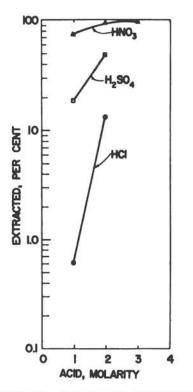
FIGURE 45. EXTRACTION OF URANIUM WITH TRI-N-OCTYLPHOSPHINE OXIDE FROM URANIUM(IV) SOLUTIONS. Uranium(IV) - 17 mg; TOPO - 0.1 M in cyclohexane, 5 ml; Phase ratiol; and Extraction time - 10 minutes.
