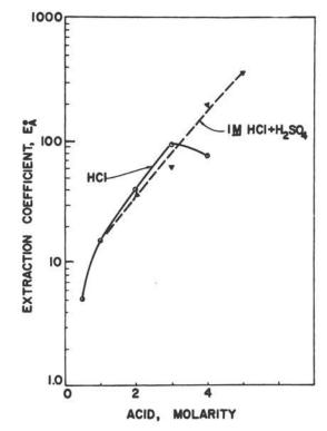
FIGURE 5. EFFECT OF ACID CONCENTRATION ON THE EXTRACTION OF ZINC WITH TRI-N-OCTYLPHOSPHINE OXIDE. Zinc - 5 mg; TOPO -0.1 N cyclohexane, 5 ml; Phase ratio - 1; and Extraction time - 10 minutes.
