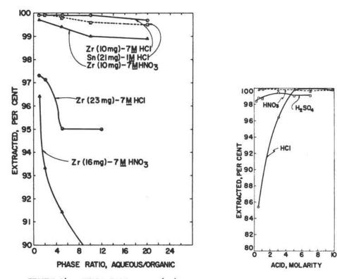
FIGURE 14. EXTRACTION OF TIN(IV) AND ZIRCONIUM WITH TRI-N-OCTYL-PHOSPHINE OXIDE AS A FUNCTION OF EXTRACTION TIME. TOPO, 0.1 M in cyclohexane, 5 ml; and Extraction time - 10 minutes.
