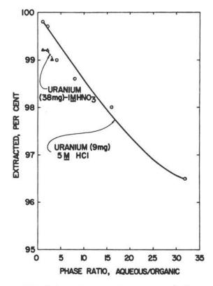
FIGURE 17. EXTRACTION OF URANIUM(VI) WITH TRI-N-OCTYLPHOSPHINE OXIDE AS A FUNCTION OF PHASE RATIO. TOPO - 0.1 M in cyclohexane, 5 ml and Extraction time - 10 minutes.
