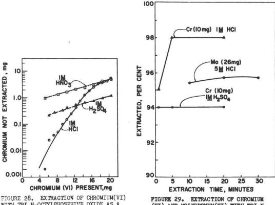
WITH TRI-N-OCTYLPHOSPHINE OXIDE AS A FUNCTION OF CHROMIUM CONCENTRATION. TOPO - 0.1 <u>M</u> in cyclohexane, 5 ml; Phase ratio - 1; and Extraction time - 10 minutes.
