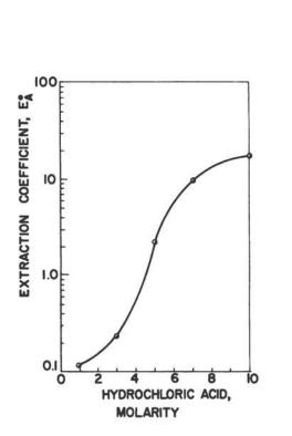
FIGURE 20. EXTRACTION OF ARSENIC(III) WITH TRI-N-OCTYLPHOSPHINE OXIDE AS A FUNCTION OF HYDROCHLORIC ACID CONCEN-TRATION. Arsenic(III) - 1.0 mg; TOPO -0.1 M in cyclohexane, 5 ml; Phase ratio -1; and Extraction time - 10 minutes.
