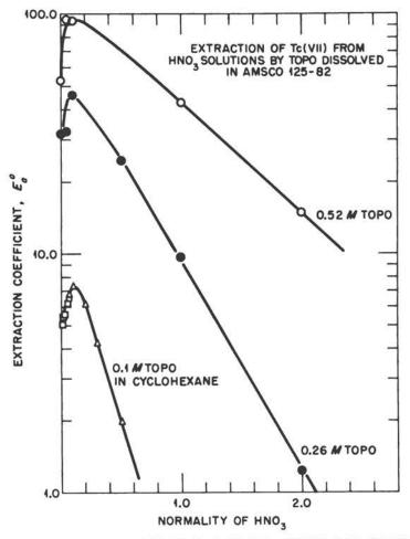
FIGURE 32a. EXTRACTION OF TECHNETIUM FROM NITRIC ACID SOLUTIONS WITH CYCLOHEXANE SOLUTIONS OF TRI-N-OCTYLPHOSPHINE OXIDE
