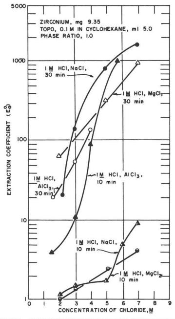
FIGURF 9. EXTRACTION OF ZIRCONIUM BY 0.1 M TRI-N-OCTYLFHOSPHINE OXIDE AS A FUNCTION OF THE CONCENTRATION OF CHLORIDE SALTS OF UNI-, DI-, AND TRI-VALENT METALS
