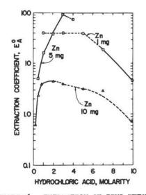
FIGURE 6. EXTRACTION OF ZINC WITH TRI-N-OCTYLPHOSPHINE OXIDE AS A FUNCTION OF HYDROCHLORIC ACID CONCEN-TRATION. TOPO - 0.1 M cyclohexane, 5 ml; Phase ratio - 1; and Extraction time - 10 minutes.
