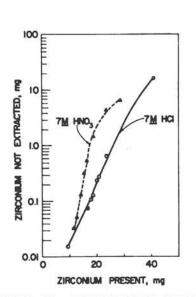
FIGURE 12. EXTRACTION OF ZIRCONIUM WITH 0.1 M TRI-N-OCTYLPHOSPHINE OXIDE. TOPO - 0.1 M in cyclohexane, 5 ml; Phase ratio - 1; and Extraction time -10 minutes.
