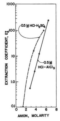
FIGURE 23. EFFECT OF CHLORIDE AND SULFATE ON THE EXTRACTION OF ANTIMONY (V) FROM CHLORIDE SOLUTIONS WITH TRI-N-OCTYLPHOSPHINE OXIDE. Antimony -9 mg; HCl - 0.5 M; TOPO - 0.1 M in cyclohexane, 5 ml; Phase ratio - 1; and Extraction time - 10 minutes.
