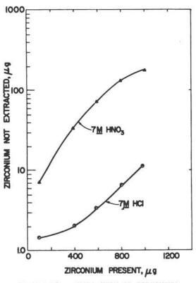
FIGURE 13. EXTRACTION OF ZIRCONIUM WITH 0.01M TRI-N-OCTYLPHOSPHINE OXIDE. TOPO - 0.1 M in cyclohexane, 5 ml; Phase ratio - 1; and Extraction time -20 minutes.
