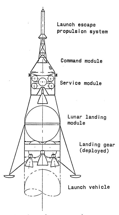
Figure 1. - General arrangement - lunar landing configuration.
