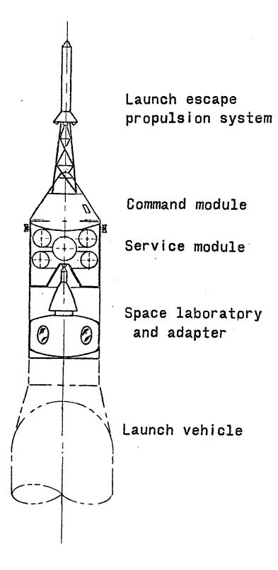
Figure 2. - General arrangement - earth orbital configuration with space laboratory.
