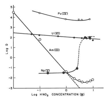
Fig. 12. Extraction of various actinides into 0.5  $\underline{\rm M}$  HDEHP (isooctane diluent) from HNO\_3 solutions.^{238}
