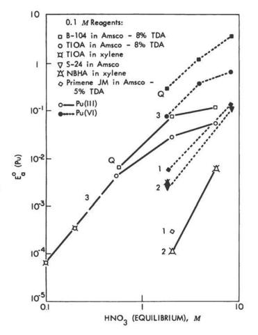
Fig. 23. Pu(III) and Pu(VI) extraction by 0.1 <u>M</u> amines: effect of nitric acid concentration. Amine class: (Q) quaternary ammonium. (3) tertiary, (2) secondary, (1) primary amine. Pu reduced with 0.03 <u>M</u> ferrous sulfamate plus 0.05 <u>M</u> excess sulfamic acid, or oxidized with AgO.<sup>187</sup>
