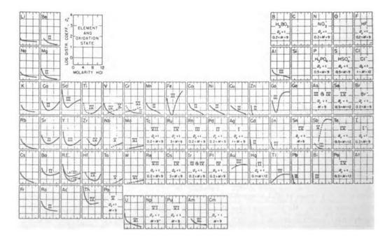
Fig. 42. Volume distribution coefficient of the elements vs HCl concentration for Dowex 50  $\times$  4 cation exchange resin. Tracer concentrations of the elements were used for the most part.  $^{300}$
