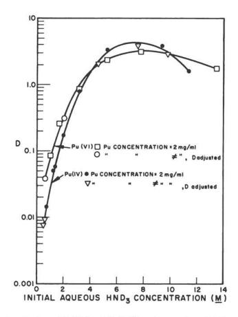
Fig. 32. Distribution of Pu(IV) and Pu(VI) into hexone from HNO<sub>3</sub> solutions.<sup>260</sup>
