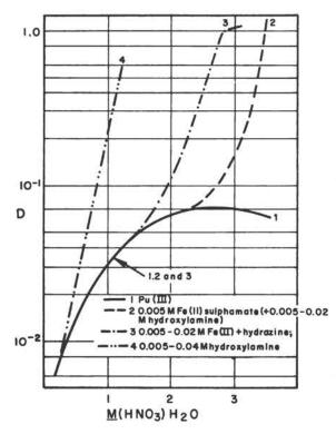
Fig. 2. Distribution of Pu(III) and equilibrium Pu(III), Pu(IV), and Pu(VI), mixtures in the presences of several reducing agents in 40% TBP in kerosene and nitric acid: after Carleson.<sup>76</sup>
