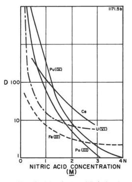
Fig. 43. Distribution of Pu(III) and Pu(IV) and other ions between nitric acid solutions and the cation resin C·50 (similar to Dowex-50).<sup>325</sup>
