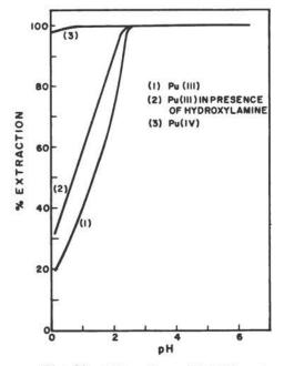
Fig. 38. Extraction of Pu(III) and Pu(IV) from 1.0 M chloride into cupferron-CHCl<sub>3</sub>. 220 Curve 1: Pu(III) = 2.16 × 10<sup>-3</sup> M, cupferron = 3.98 × 10<sup>-2</sup> M; Curve 2: Pu(III) = 3.65 × 10<sup>-3</sup> M; cupferron = 3.68 × 10<sup>-2</sup> M, 10 w/v% hydroxylamine hydrochloride. The curves are % extraction for equal phase volumes vs equilibrium pH.
