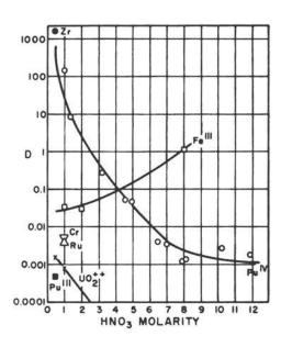
Fig. 37. Distribution coefficients of various ions from nitric acid solutions into 0.2  $\underline{M}$  TTA in benzene.<sup>110</sup>.111
