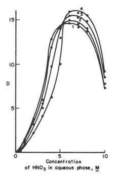
Fig. 3. Dependence of distribution coefficient of Pu(IV) into TBP on concentration of nitric acid in aqueous phase (for 281 solutions not containing uranyl nitrate). Curve 1-20°, curve 2-30°, curve 3-50°, and curve 4-70°.
