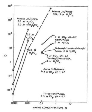
Fig. 29. Extraction of Pu(IV)from sulfuric acid and acidic sulfate solution by primary, secondary, and tertiary amines. Diluents: xylene, Amsco 125-82, or 95% Amsco 125-82-5% tridecanol. For primary amine extraction, Pu reduced with hydroxylamine sulfate, reoxidized and stabilized at (IV) with 0.5 <u>M</u> NaNO<sub>2</sub>. Others stabilized at (IV) with 0.1-0.5 <u>M</u> NaNO<sub>2</sub>.<sup>187</sup>
