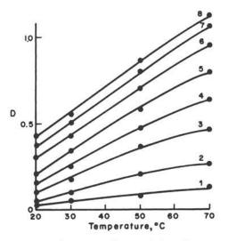
Fig. 5. Dependence of distribution cocfficient of Pu(IV) into TBP on temperature with a uranium content of 0.42 M in the aqueous phase.<sup>281</sup> Concentration of HNO<sub>3</sub>: curve 1-0.5N, curve 2-1N, curve 3-2N, curve 4-3N, curve 5-4N, curve 6-6N, curve 7-8N, and curve 8-10N.
