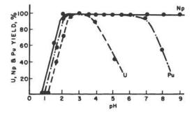
Fig. 56. Relation of element yield to solution pH. The current density on the cathode was 100 mA/cm<sup>2</sup> and the electrolysis time, 2 hr. The solution was nitric acid.<sup>344</sup>
