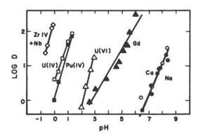
Fig. 47. Log D for some metal ions as a function of pH on silica gel (KEBO, 50-100 mesh). $^{22}$
