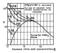
Fig. 7. Effect of NaNO<sub>3</sub> on the distribution of Pu(IV) between 19% TBP in kerosene and nitric acid solutions.<sup>44</sup>, 258
