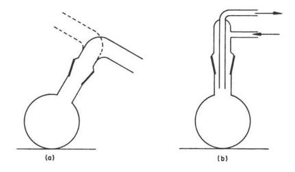
Fig. 59. Roundbottom flask used for destruction of organic matter. (a) Set-up used for refluxing (----) and removal (---) of nitric acid. (b) Set-up used for removing chloroform and sulfur-trioxide vapors.
