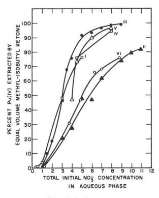
Fig. 33. Effect of total nitrate ion concentration on the extraction of Pu(IV) by methyl isobutyl ketone.<sup>393</sup>
