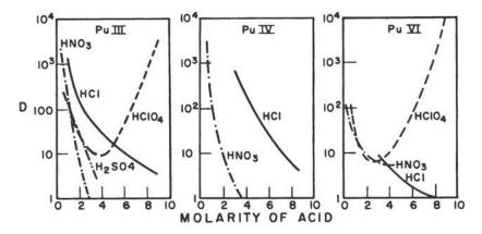
Fig. 39. Typical distribution coefficients of Pu on Dowex 50 in common acidic solutions.
