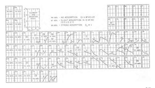
Fig. 54. Adsorption of the elements from hydrochloric acid solution by Dowex 1.240
