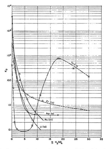
Fig. 50. Absorption of various actinide ions from  $H_2SO_4$  solutions by Dowex 2.<sup>433</sup>
