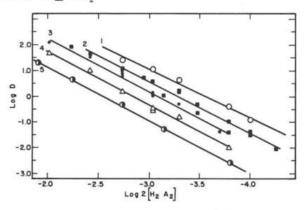
Fig. 14. Variation of the distribution coefficient of Pu(IV) as a function of the concentration of the dimer,  $(HDBP)_2$  in benzene.<sup>121</sup>  $HNO_3 + NaNO_3 = 6 M$ ;  $HNO_3$  concentrations:
