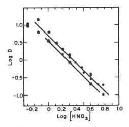
Fig. 15. Variation of the distribution coefficient of Pu(IV) from nitrate solutions by HDBP as a function of  $HNO_3$  concentration.<sup>121</sup>
