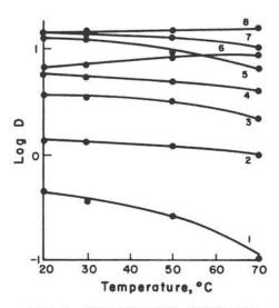
Fig. 4. Dependence of distribution coefficient of Pu(IV) into TBP on temperature in solutions not containing uranium.<sup>281</sup> Concentration of HNO<sub>3</sub>: curve 1-0.5N, curve 2-1N, curve 3-2N, curve 4-3N, curve 5-4N, curve 6-10N, curve 7-5N, and curve 8-6 to 8N.
