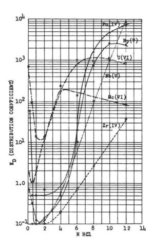
Fig. 48. Equilibrium distribution coefficients for Dowex 2 in HCl solutions.  $^{432, 433}$  (Mo, Zr, and Nb curves furnished by L. R. Bunney et al.  $^{68}$
