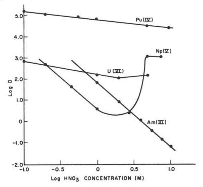
Fig. 17. Extraction of various actinides into 0.2  $\underline{M}$  H<sub>2</sub>MEHP (isooctane diluent) from HNO<sub>3</sub> solutions.<sup>238</sup>
