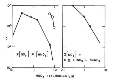
Fig. 13. Pu(IV) extraction by di(2-ethylhexyl)-phosphoric acid: effect of nitric acid and sodium nitrate concentration.  $\bigcirc$  0.01 <u>M</u> D2EHPA:  $\bigcirc$  0.1 <u>M</u> D2EHPA; diluent, Amsco 125-82. Plutonium reduced with hydroxylamine nitrate, reoxidized and stabilized with 0.1-0.5 <u>M</u> NaNO<sub>2</sub>.<sup>187</sup>
