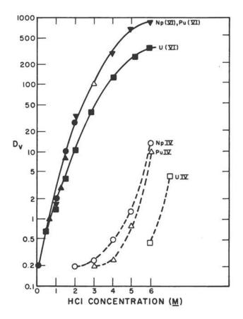
Fig. 52. Volume distribution coefficients, Dv, for tetra and hexavalent U, Np, and Pu between Dowex 1 and hydrochloric acid solutions.  $^{266}$
