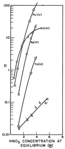
Fig. 34. Extraction of actinides and Zr by 1.09 <u>M</u> N, N-dibutyloctanamide in n-dodecane at 30°. 378
