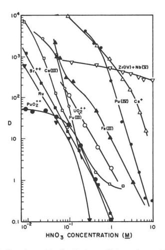
Fig. 46. The dependence of the distribution coefficients of several ions on zirconium phosphate on the aqueous  $HNO_3$  concentration. All adsorbates present in tracer amounts. Solutions of Pu(III) were 0.005 <u>M</u> in sulphamic acid and 0.015 <u>M</u> in hydrazine; solutions of Pu(IV) 0.02 <u>M</u> in NaNO<sub>2</sub> and solutions of  $PuO_2^{++}$  0.02 <u>M</u> in KBrO<sub>3</sub>.<sup>140</sup>
