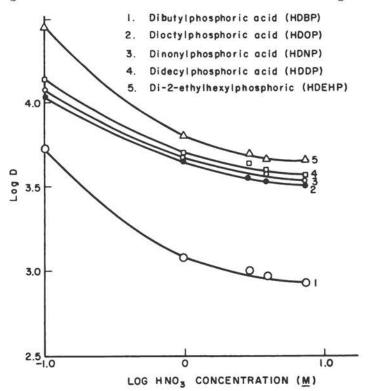
Fig. 11. Extraction of Pu(IV) by dialkylphosphoric acids (0.5  $\underline{M}$  in isooctane) from HNO<sub>3</sub> solutions.<sup>238</sup>
