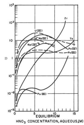
Fig. 1. Extraction of nitrates at trace concentration into 19 volume % TBP in kerosene at 25°C from nitric acid solutions. Taken from McKay and Healy.<sup>259</sup> The individual references are: yttrium<sup>350</sup>; thorium <sup>179</sup>; zirconium<sup>25</sup>; uranium and neptunium<sup>26</sup>; and plutonium<sup>44</sup>, 258.
