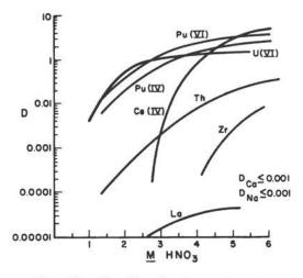
Fig. 30. The distribution ratios of U, Pu(IV) and Pu(VI), Th, Zr, Ce(IV) and La into hexone as functions of the equilibrium concentration of HNO<sub>3</sub> in the aqueous phase.<sup>343</sup> The Ce(IV) curve is taken from Glendenin <u>et al.</u><sup>147</sup>
