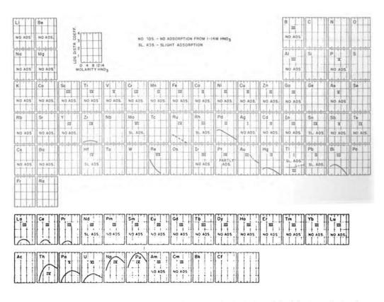
Fig. 55. Removal of elements from solution in 1  $\underline{M}$  nitric acid with strongly basic anion-exchange resin.<sup>127</sup>
