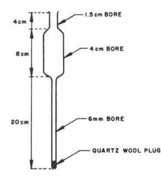
Fig. 60. Ion exchange column.
