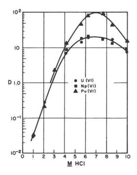
Fig. 28. Extraction of hexavalent U, Np, and Pu from HCl solution with 1.0% TOA in xylene.<sup>217</sup>
