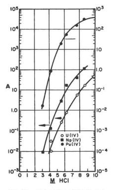
Fig. 27. Extraction of U(IV) and Np(IV) by 10% TOA and Pu(IV) by  $1\cdot0\%$  TOA from HCl solutions.<sup>217</sup>
