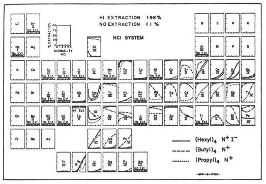
Fig. 26. Extraction of elements as tetraalkyl amine complexes from hydrochloric acid.  $^{262}$
