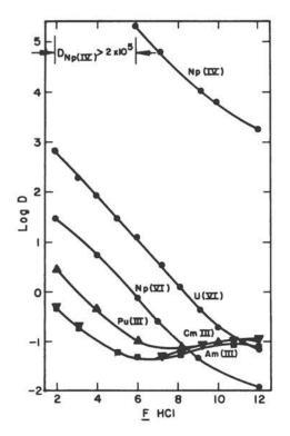
Fig. 18. Extraction of some actinide cations into 0.48 F  $H_2MEHP$  in toluene as a function of HCl concentration.<sup>313</sup>
