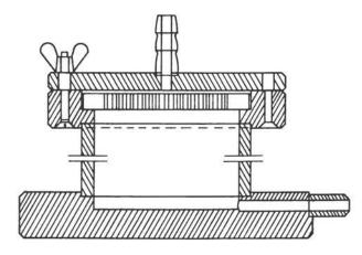
Fig. 58. Cross sectional view of the agitation column. The material is "Altuglas MZD" throughout except for the brass screws. The diffuser plate has a total of 213 holes drilled on 8 concentric circles. The inside dimensions of the column are 8.0 cm diameter by 60 cm high. The reader is referred to the original paper for a more detailed drawing.
