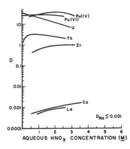
Fig 31. The distribution ratios of U. Pu(IV) and Pu(VI). Th, Zr, La and Ca into hexone as functions of the equilibrium concentration of  $HNO_3$  in the aqueous phase. Concentration of  $Ca(NO_3)_2$  4-3.5 <u>M</u>.<sup>343</sup>
