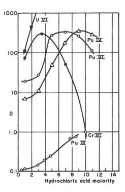
Fig. 10. Extraction of metal ions from hydrochloric acid by 0.1  $\underline{M}$  TOPO in cyclohexane.<sup>269</sup>
