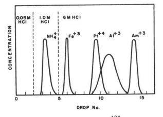
Fig. 45. Separation of Am from some common impurities by elution with HCl. The abcissa is drop number for a 0.3-cm diameter by 10-cm column. The resin used was Dowex  $50 \times 4$ .
