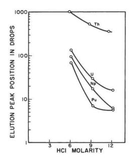
Fig. 41. Elution peak position of the tetrapositive ions vs hydrochloric acid molarity.  $^{117}\,$
