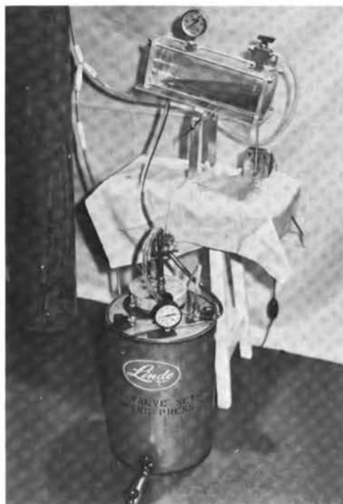
FIGURE 2. Portable assembly showing oxygen tank, oscillating 1-liter pressurized chamber containing blood for perfusion of the organ, and stainless-steel cylinder (which is pressurized to 54 psig).
