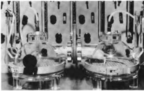
FIGURE 2. Method of transferring rat into a clean chamber. Chamber on the right is disconnected for cleaning. (Reproduced from Aerospace Med. 37:243, 1966.)
