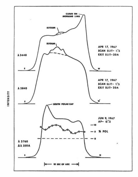
FIGURE 5 Scans of Mars near its 1967 opposition. The upper two curves are area scans made by Boyce in the E-W direction through Elysium. A spectral scanner was used to limit the wavelength band under observation. The solid curve at the bottom is one of eight intensity scans made by Hall in a N-S direction with a polarimeter. The resulting polarization is shown by the open circles.
