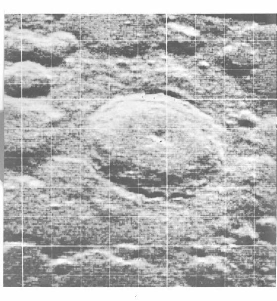
Map of the radar reflectivity at 3.8-cm wavelength for the region surrounding the lunar crater Tycho, made by the Haystack Microwave Facility. Surface resolution is approximately 1 km. (Courtesy MIT Lincoln Laboratory)
