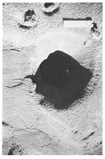
Figure 32. Close-up of a sandboil. Note small slide-rule for scale.
