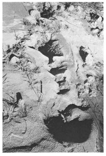
Figure 31. Detail of the sandboils shown in Figure 30. Note pen for scale.
