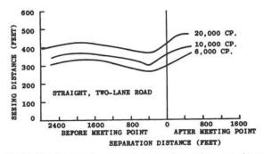
Figure 2—Visibility distance in a two-lane road meeting as a function of candlepower at ½ °D-2 °R. (Data from Roper and Meese, 1964.)
