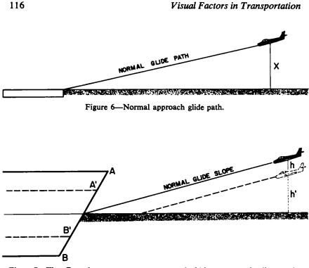
Figure 7—The effect of a narrower versus a normal width runway on landing an aircraft. AB is the width of a normal runway; A'B' is the width of a narrow runway; h' is the height for a narrow runway; h + h' is the height for a normal runway. At the same point in the approach the pilot feels as though h' is equal to h + h'. A normal glide path at height h' results in the tendency to undershoot or land short of the runway.
