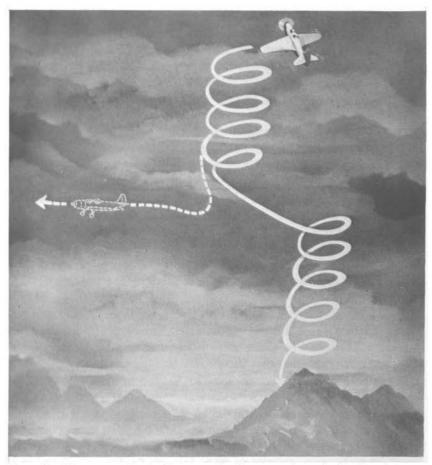
Figure 2—The graveyard spin. In recovering from a prolonged spin, the pilot perceives the start of a spin in the opposite direction. (The dotted line indicates perceived motion; the solid line shows actual motion.) Correcting for this impression, he goes into another spin in the original direction.
