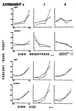
Figure 4—Visibility effects of brightness (upper) and size (lower) of simulated green signs, observed (dotted) and calculated values. (Day and night alternately from top). Experiments, 6, bright letters; 7, blank; 8, letter brightness reduced on darker signs. From Forbes *et al.*, 1968.
