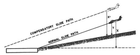
Figure 12—The effect of terrain upslope on the aircraft glide slope. When there is an upslope in the runway approach zone, the aircraft appear to be above normal glide path. To compensate, the pilot would fly a glide slope that results in a long landing.
