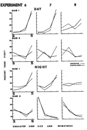
Figure 5-Visibility effects of size and brightness varied together (top) and oppositely (second row). Observed (dotted) and calculated. From Forbes et al., 1968.
