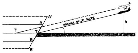
Figure 8—The effect of a wide runway versus a normal width runway on aircraft landing. AB is the width of a normal runway; A'B' is the width of a wide runway; h is the height for a normal runway; h' + h is the height of aircraft for a wider runway. At the same point in the approach, h + h' is thought by the pilot to be equal to h. Thus, the aircraft's normal glide slope results in an overshoot or landing too far down the runway.
