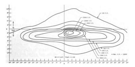
Figure 1-Isocandlepower diagram of 53/4", type-2 low beam, headlamp.
