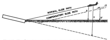
Figure 9—The effect of runway upslope on glide path. When the runway has an upsolpe, the normal glide path will seem too steep. Flying in glide path that appears more normal could result in a landing short of the runway.
