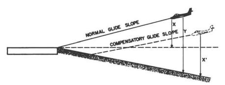
Figure 10—The effect of terrain downslope in the runway approach on aircraft glide path. With a terrain downslope, the pilot will believe the aircraft to be on low, flat approach, and there is a tendency to land short of the runway.
