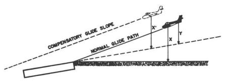
Figure 11—The effect of runway downslope on the aircraft glide path. When the runway has a downslope, the normal glide path will appear flat, and there is a tendency to overshoot.
