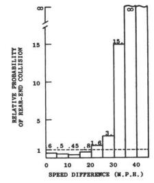
Figure 10-The effect of relative velocity upon rear-end collision probability.
