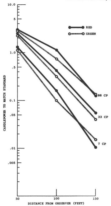
Figure 15—Perceived intensities of red and green-blue lights at three distances in a 200' night fog.
