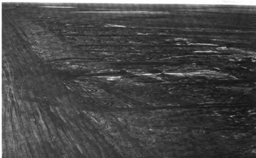
FIGURE 8 Oblique view of terrain disturbance on north of airstrip at Sachs Harbour, southwest Banks Island. The raised sections were used to transport material from the intervening depressions to the airstrip; 25 July 1971.
