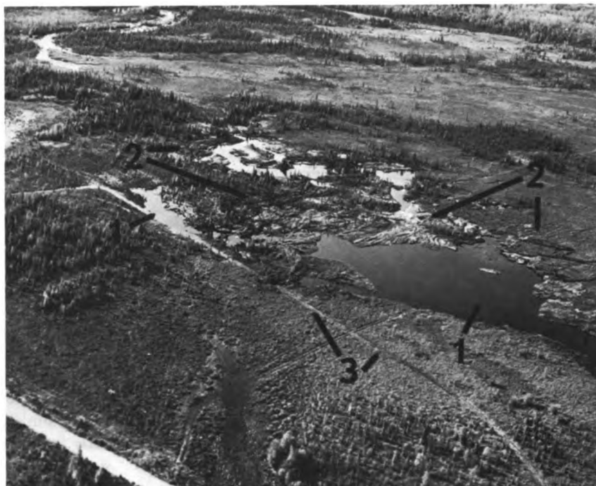
FIGURE 5 Aerial view of pond and rolled and compressed vegetation and organic layers caused by the 1967 flood. (1) Pond areas that were bog and black spruce muskeg before the flood; (2) areas of compressed vegetation; and (3) old vehicle trails that may have caused break in vegetation mat.
