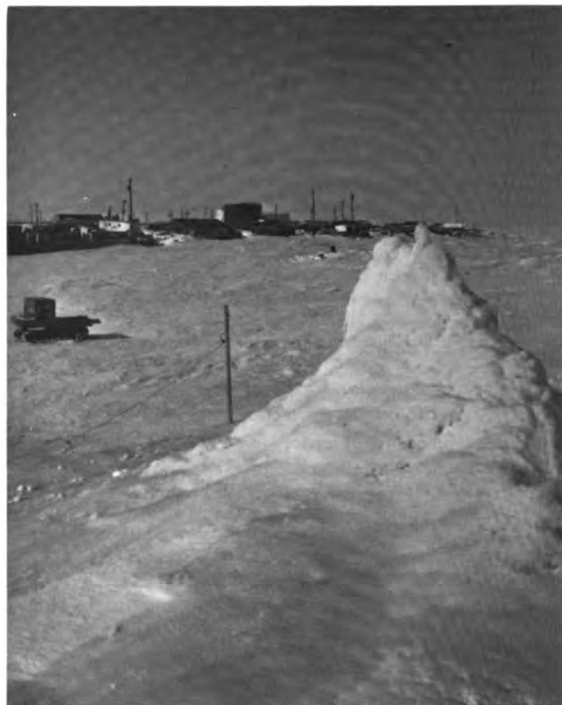
FIGURE 1 Artificially grown ice mound produced near Kotzebue, Alaska, in 1966 as a part of University of Alaska, Arctic Environmental Engineering Laboratory studies. A small pump with hose and discharge nozzle was used to pump saline water that was desalinated by freezing as the water traveled through subzero air to storage in the ice mound. 1
