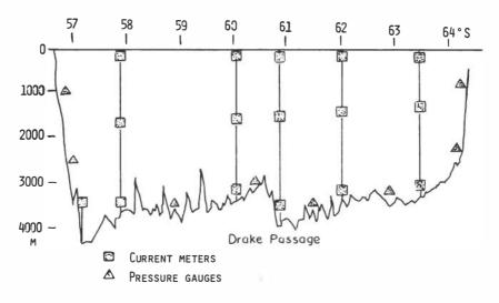
FIGURE 3.3 Recommended eventual arrangement of instruments across the Drake Passage; the first long-term moorings would involve fewer instruments.
