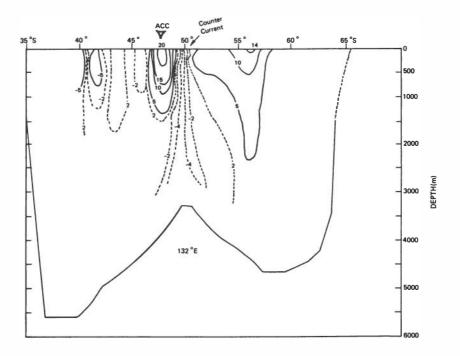
FIGURE 3.2 Zonal component of absolute velocity (in centimeters/second, positive east) at 132° E. Vertical exaggeration is 500 [J. E. Callahan, *J. Geophys. Res. 76*, 5860, 1971. Copyright by American Geophysical Union.]
