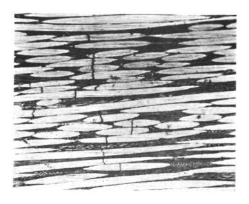
Fig. 7 - Close-up of longitudinal section of CFRP showing fibres cracked during a fatigue test
