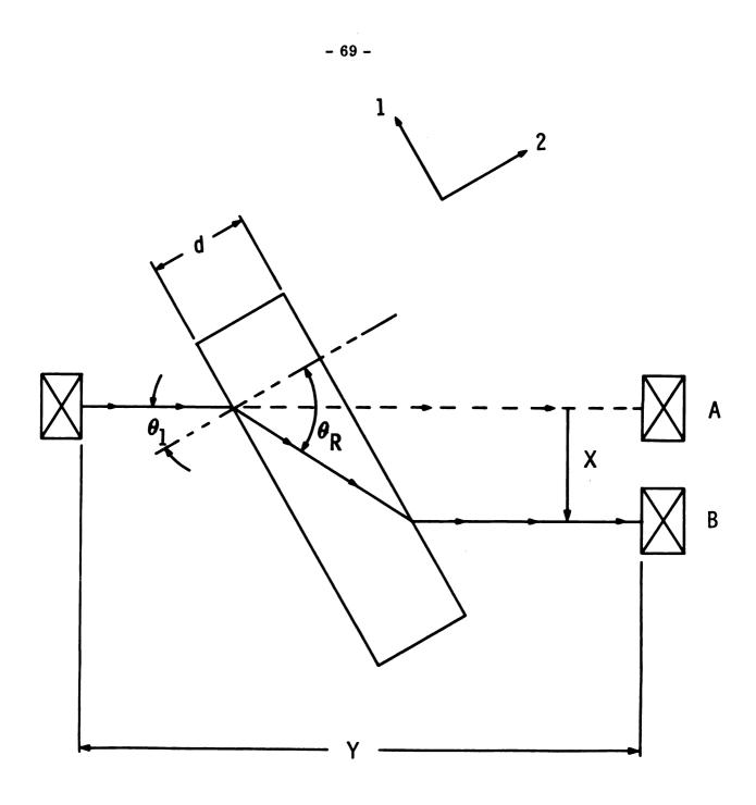
Fig. 1° - Composite material property determination with ultrasonics
