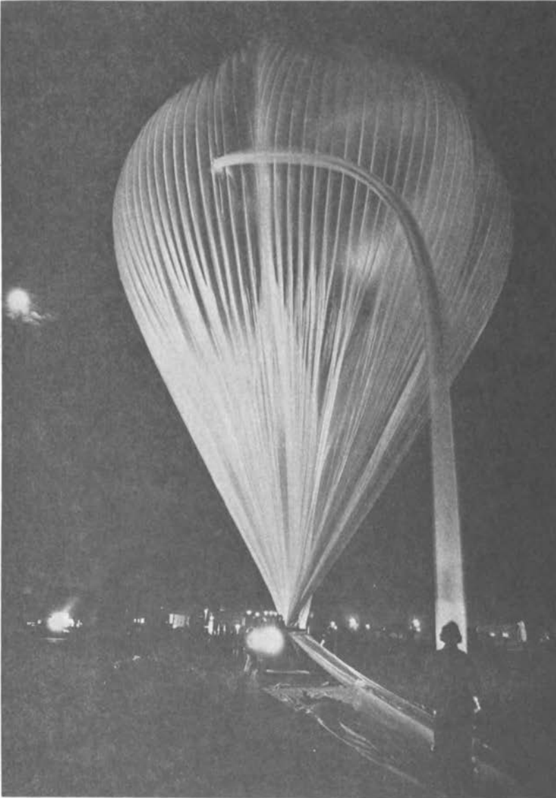
FIGURE A.1 A large balloon being inflated in preparation for launching a Washington University cosmic-ray package. (Photograph courtesy of Richard N. Levine, Washington University, St. Louis.)
