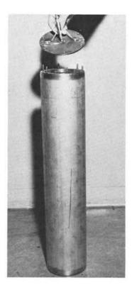
FIGURE 13 Stainless steel capsules with metal gaskets and bolted closures are used at the Oak Ridge National Laboratory for storage of small packages of transuranium-contaminated waste containing high-radiation-level gamma emitters. The capsules are stored in stainless-steel-lined wells with concrete shielding plug closures.
