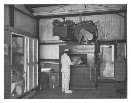
FIGURE 5 Operation of a 50-ton hydraulic solid waste compactor at the Idaho National Engineering Laboratory reduces the waste volume by a factor of 10 to 1 and produces 0.4-cubic-meter (14-cubic-foot) bales averaging 270 kilograms (600 pounds) contained in plastic-lined cardboard boxes. Only waste with low levels of beta-gamma contamination is processed in this way.
