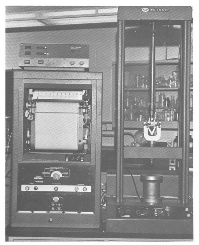
FIGURE 2 Instron Universal Testing Machine with Warner-Bratzler attachment.
