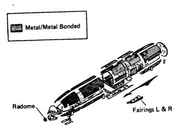
Figure 1. Structural Bonding-Fuselage
