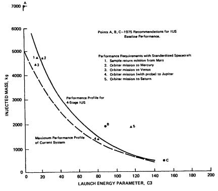
FIGURE 1 Performance profile for current and IUS launch systems.
