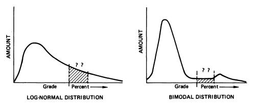
FIGURE 4.5 Possible distribution of mineral materials in the earth's crust. (A basic question is the distribution of materials in the shaded area.)
