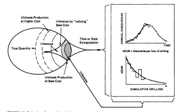
FIGURE 4.3 Estimation of potential supply by time and rate methods.
