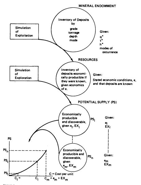
FIGURE 4.12 A potential supply system (model).
