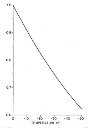
FIGURE B.2 Water activity  $a_w = p_{ice}/p_{H_2O}$  of a solution in equilibrium with ice as a function of temperature.
