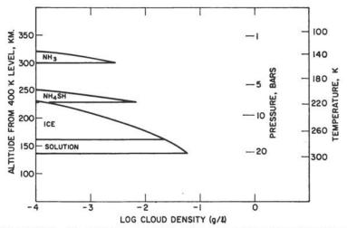
FIGURE C.3.2 Nominal Saturn model, solar composition. Note change in vertical scale.
