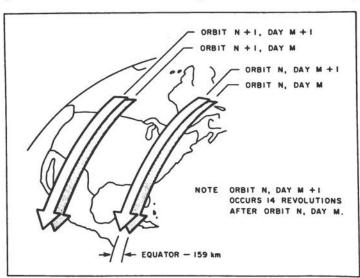
FIGURE 20 Landsat orbits repeat on an 18-day cycle. Adjacent swaths on adjacent days overlap some 15 percent near the equator; the overlapping becomes progressively larger at higher latitudes.
