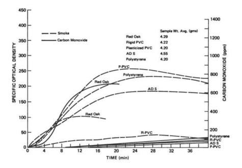
Figure 5. Smoke and carbon monoxide from various materials, average of triplicate tests smoldering exposure (2.00 w/cm<sup>2</sup>). (57)
