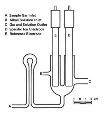
Figure 10. HCN monitoring device (73).
