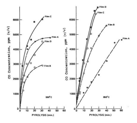
Figure 13. Generation of carbon monoxide in pyrolysis of 5<sub>g</sub> film samples at 550°C and 650°C. (102)
