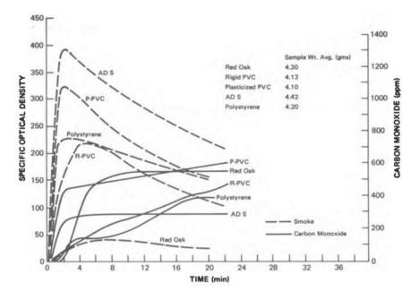
Figure 6. Smoke and carbon monoxide from various materials, average triplicate tests flaming exposure (2.00 w/cm<sup>2</sup>). (57)
