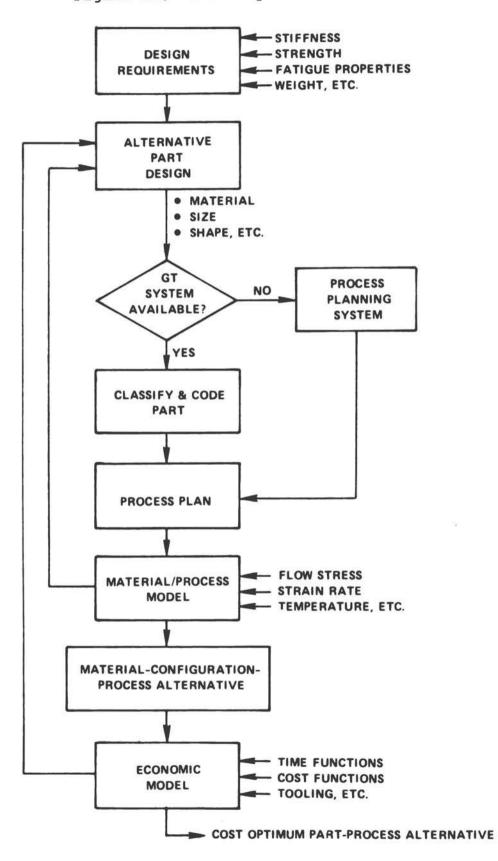
Figure 11. Basic system structure
