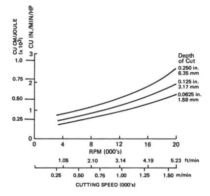
Figure 1. Effect of cutting speed on metal removal efficiency for aluminum alloy blocks milled to various depths with two-flute, 0.5 in. diameter carbide cutters<sup>3</sup>.
