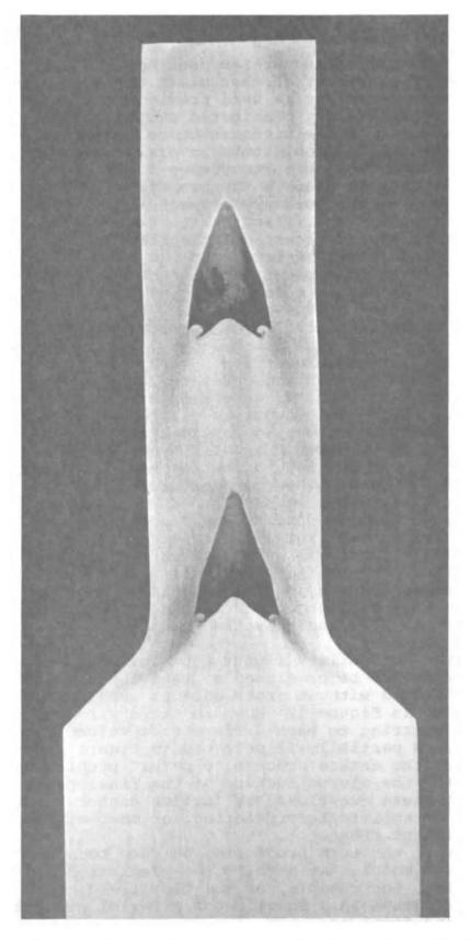
Figure 1. Illustration of central burst fracture during extrusion
