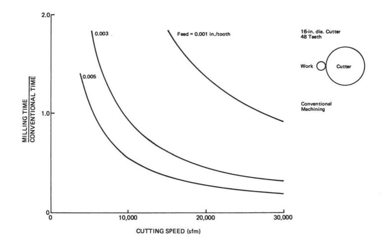
Figure 3. Effect of cutting speed on the ratio of milling time to conventional time as a function of feed/tooth for machining a steel automotive reverse sun transmission gear tool forces encountered would be anticipated to decrease the level of induced residual stress and eliminate the need for post-machining stress relief heat treatments.
