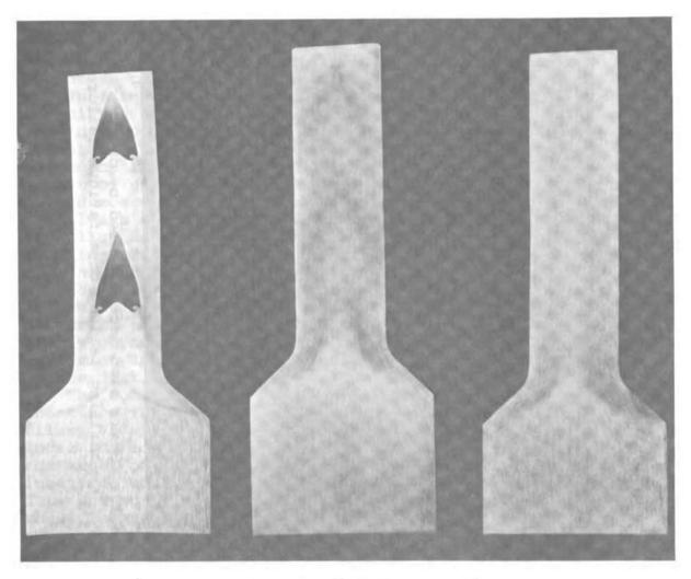
Figure 9. Shear band defect leading to an extrusion center burst
