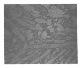
Figure 4. Primary alpha plus transformed beta Ti-6242 microstructure
