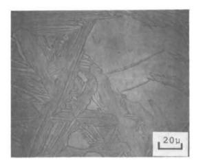
Figure 3. Widmanstatten or transformed beta Ti-6242 microstructure
