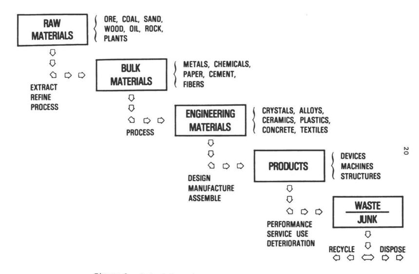
Figure 3. Materials and processing sequence
