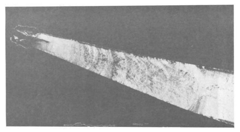
Figure 10. Shear band defect caused by die chilling leading to a fatigue failure
