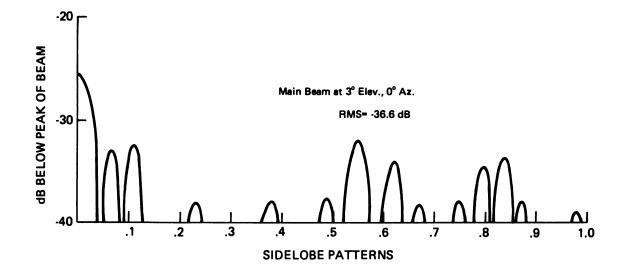
Figure 5 Calculated Radiation Intensity During Enhanced Search Courtesy of the United States Air Force
