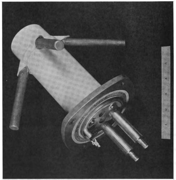
Figure 3 PAVE PAWS Radar Antenna Element Courtesy of the United States Air Force
