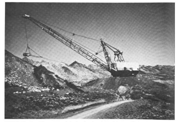
FIGURE 10 Dragline on an interburden bench casting spoil to its right.
