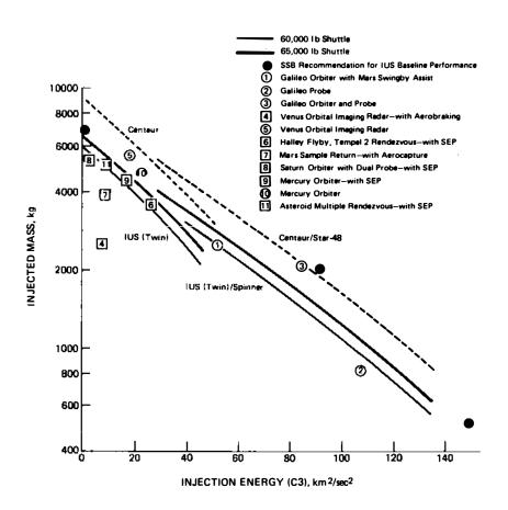
FIGURE 1 The heavy line indicates the capability of the nominal Shuttle-IUS performance, due to be available after 1984; the light line indicates performance planned for 1984. Also shown are performance requirements for several selected mission possibilities with indicated assumptions about technological developments. Numbered circles rely on present technology used with Shuttle-IUS; numbered squares assume new technological development in spacecraft propulsion.
