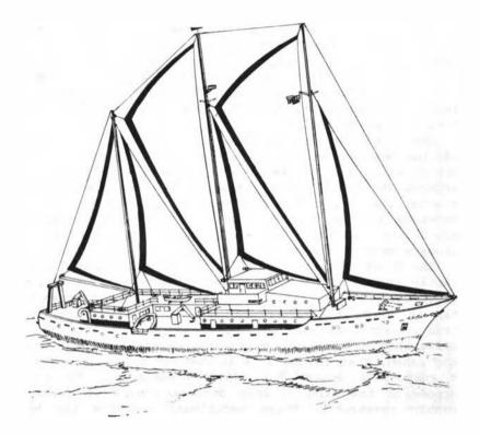
FIGURE 2 Design sketch of oceanographic motor-sailer.
