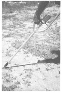
Several inexpensive tools have been developed for spot seeding. Most have a device for baring mineral soil and a mechanism for metering a predetermined number of seeds onto the prepared spot. Shown is the "Panama seeding hoe." The hoe at the bottom is used to rake away litter. The trigger is then squeezed and the seeds drop down the tube onto the exposed mineral soil. The operator then normally presses the seeds into the soil with his foot as he passes to the next spot.
