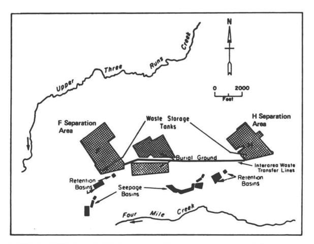
FIGURE 6 Relative locations of separation areas and associated waste-handling facilities.
