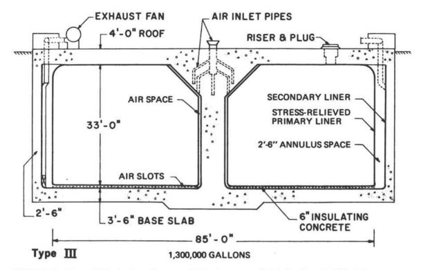
FIGURE 4 Type III tanks for cooled storage of high-level liquid radioactive waste at SRP.
