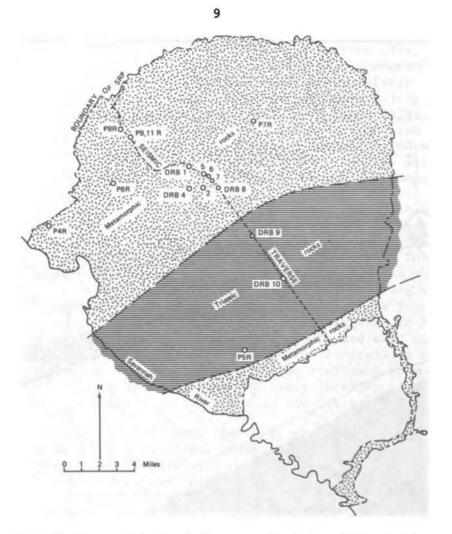
FIGURE 2 Distribution of bedrock types underlying SRP, showing location of deep rock boring sites (DRBl through DRBl0) and orientation of vertical geologic cross section (Figure 3).
