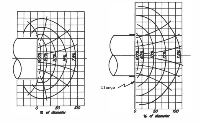
FIGURE 3-1 FIGURE 3-2 Velocity contours (expressed in percentage of opening velocity) and streamlines for circular openings. (from "Industrial Ventilation," 16th Edition, 1980)
