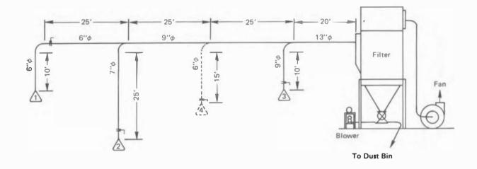
FIGURE 3-5 Typical dust-collection system.
