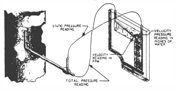
FIGURE C-4 Use of pitot tube and velometer.
