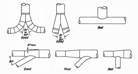
BRANCH ENTRY Branches should enter at gradual expansions and at an angle of 30° or less (preferred) to 45° II necessary.
