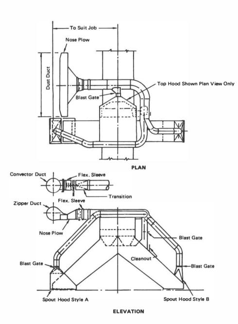
FIGURE 6-7 Zipper suction for tripper.
