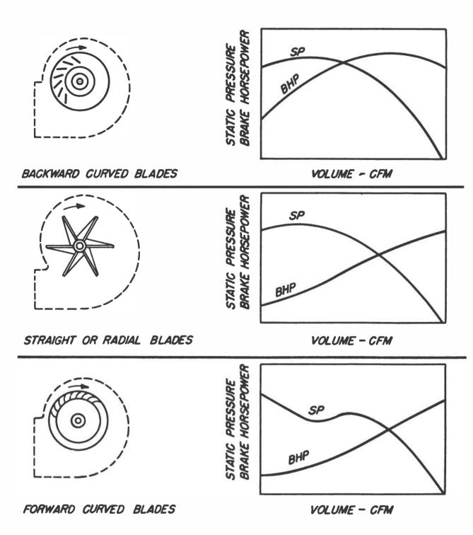
FIGURE 5-2 Centrifugal fans. (from "Industrial Ventilation", 16th Edition, 1980)
