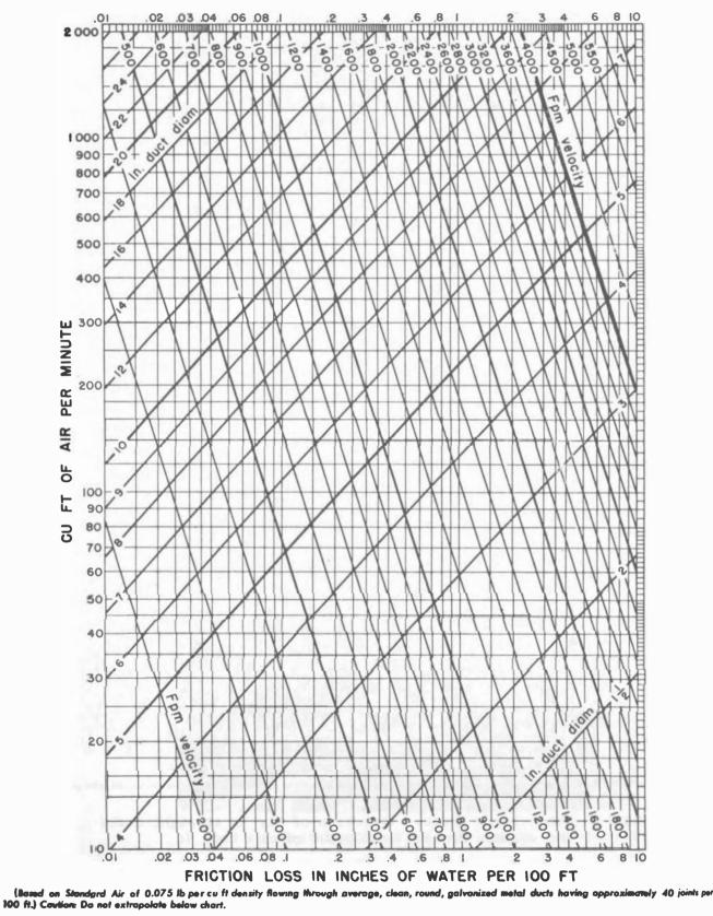
FIGURE 3-6 Tube sizing chart. (Friction of air in straight ducts for volumes of 10 to 2000 cfm.)
