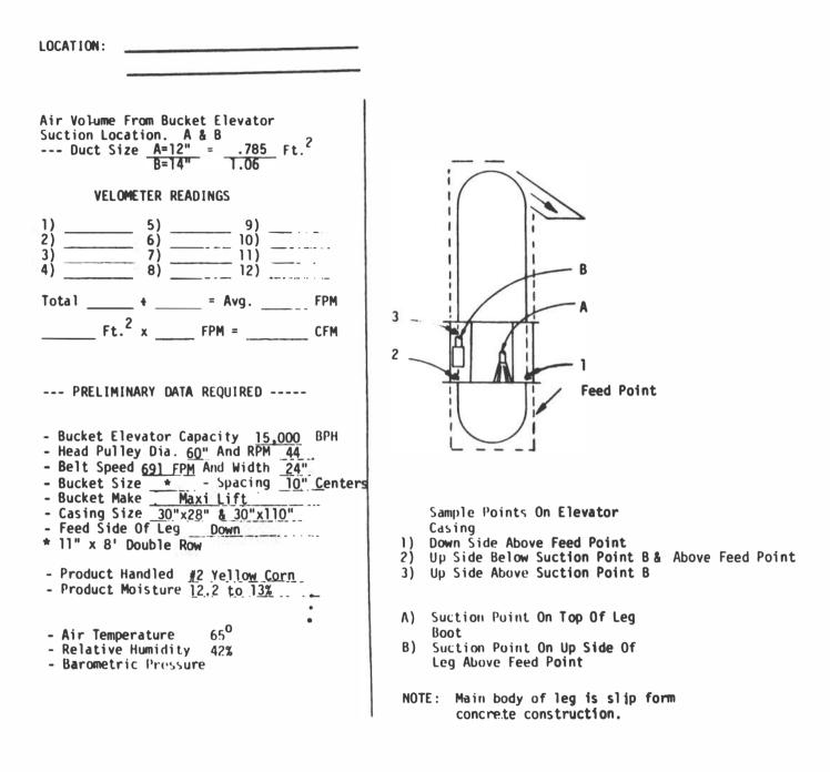
FIGURE C-1 Preliminary data sheet for a bucket elevator test.
