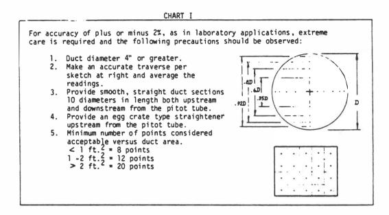
Now that we have the velocity stated in feet per minute and we have the cross sectional area of the duct stated in square feet we can multiply these two together and determine the cubic feet per minute or CFM, as we normally refer to it.
