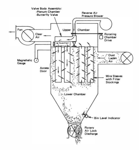
FIGURE 4-1 Typical fabric filter.
