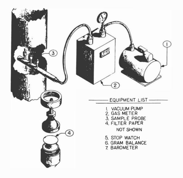
FIGURE C-2 Air flow schematic for sampling procedure.
