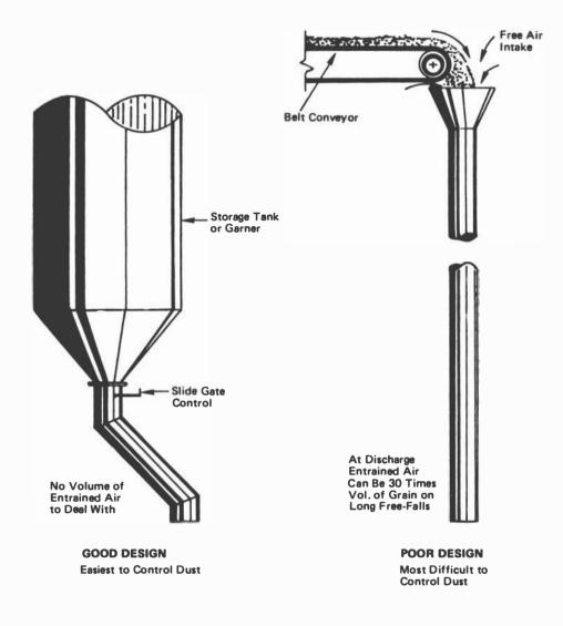
FIGURF 6-11 Load-out spout design.
