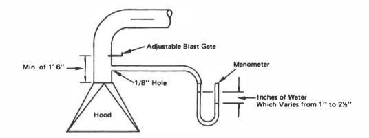
FIGURE 8-3 Typical hood and blast gate.
