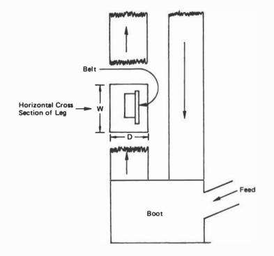
FIGURE 6-1 Rule of thumb for calculating airflow in elevator leg.
