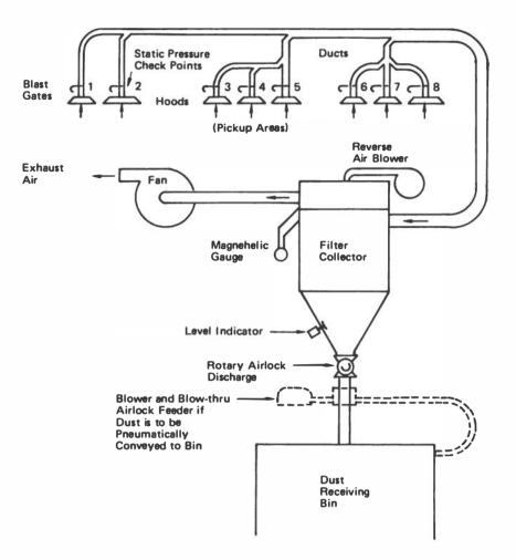
FIGURE 8-1 Typical dust control system. The figure shows an <u>exhaust</u> system because the fan draws air through the collector. If the fan is ahead (i.e., pushing air through) of the collector, it is a <u>blow</u> system. Most cyclone collectors are attached to blowing systems, and most filter collectors are attached to exhausting systems.
