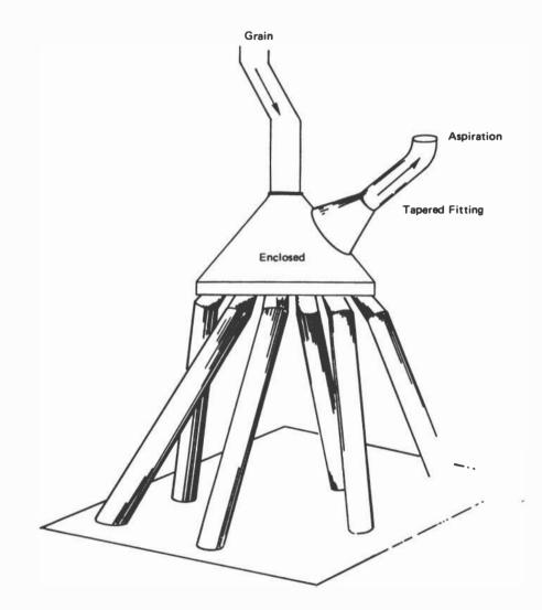
FIGURE 6-6 Enclosed distributor dust control system.
