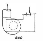
FAN INLET A straight inlet is best: if an elbow inlet is necessary, provide an inlet box and duct turn vanes to eliminate air spin or uneven loading of the fan wheel. Inlet boxes should not be used for dust - loden air.
