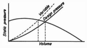
POOR SELECTION Fan with flat pressure curve gives wide volume variation with pressure change.
