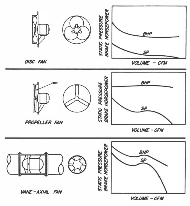
FIGURE 5-1 Axial flow fans. (from "Industrial Ventilation", 16th Edition, 1980)
