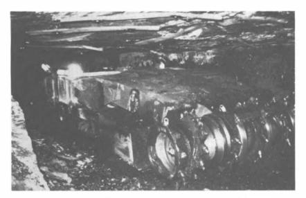
FIGURE 1 A Lee-Norse continuous miner in operation.
