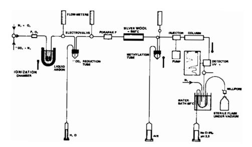
Fig. 4 Experimental setup for <sup>11</sup>C-imipramine synthesis (photograph provided by D. Comar).
