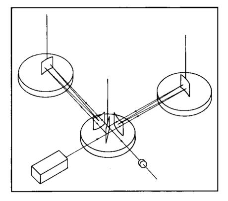
Schematic representation of a gravity wave detector based on a Michelson interferometer with multiple-reflection optical delay lines in each arm. The source of the beam, lower left, is a laser and the detector, lower right, is a photodiode. (See page 29.)
