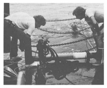
FIGURE 3.3 Launching an acoustic transponder. The acoustic package (electronics, batteries, transducer) is on deck, and the flotation units are in the water streaming astern.
