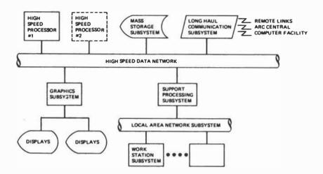
Figure 2 The NAS Processing System Network (NPSN). (Courtesy of the National Aeronautics and Space Administration.)
