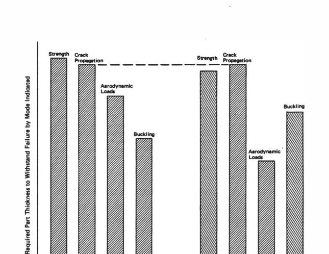
FIGURE 12 Potential weight savings considering additional failure modes (based on Ekvall 1982).
