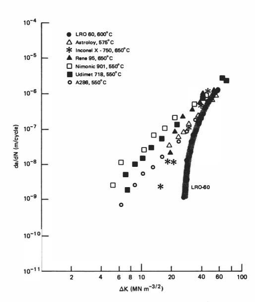
FIGURE 10 Comparison of crack growth data for LRO-60 (Fe-39.5w%Ni-22.4V-0.4Ti-0.04Ce) in high purity argon with other high-temperature alloys: Astroloy tested in high purity argon, R = 0.05, v = 10 Hz; Rene 95 tested in high purity argon, R = 0.05, v = 20 Hz (unpublished material by A. K. Kuruvilla and N. S. Stoloff, Rensselaer Polytechnic Institute, Troy, New York, 1983); Nimonic 901, Udimet 718, and A-286 tested in air at R = 0.1, v = 40 Hz (Hoffelner and Speidel 1981).
