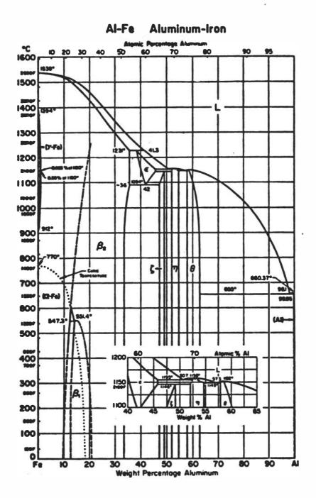
FIGURE 27 Fe-Al phase diagram (American Society for Metals 1973).
