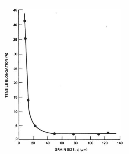
FIGURE 8 Influence of grain size on tensile ductility of NiAl at 673°K; strain rate =  $10^{-4}$  s<sup>-1</sup> (Schulson and Barker 1983).
