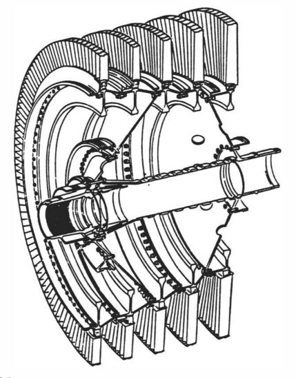
FIGURE 21 Low pressure turbine assembly of a CF6-6 engine (courtesy of General Electric Corporation).
