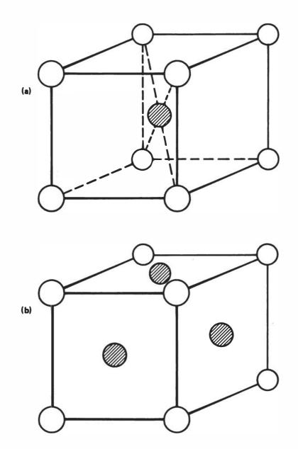
FIGURE 1 (a) At low temperatures: CuZn has the cesium chloride B2 long-range-ordered structure and (b) Cu<sub>3</sub>Au has the face centered cubic-based  $Ll_2$  structure.
