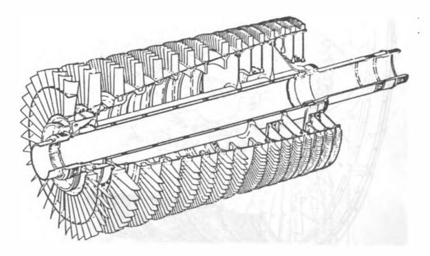
FIGURE 17 Compressor rotor of a CF6-6 engine (courtesy of General Electric Company).
