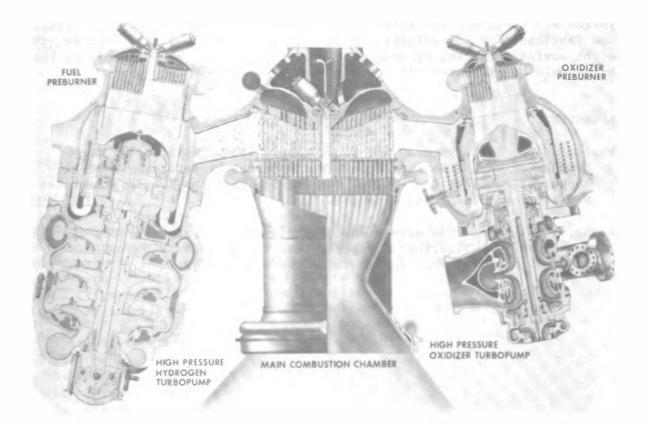
FIGURE 23 Space shuttle main engine powerhead component arrangement (courtesy of Rockwell International, Rocketdyne Division).
