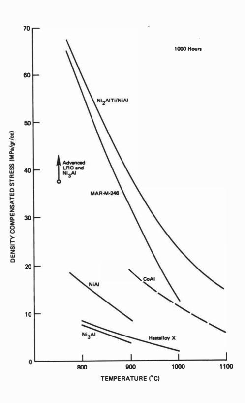
FIGURE 26 Comparative density compensated stress-rupture behavior of several alloys.
