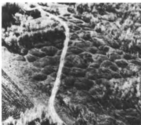
Low-angle, oblique aerial view of thermokarst mounds in an abandoned agricultural field at the U.S. Department of Agriculture Experimental Farm at the University of Alaska, Fairbanks. These mounds are located on the north-facing side of College Hill and are 10 to 30 feet in diameter. (Photograph by R.F. Black and T.L. Pévé, September 10, 1948).
