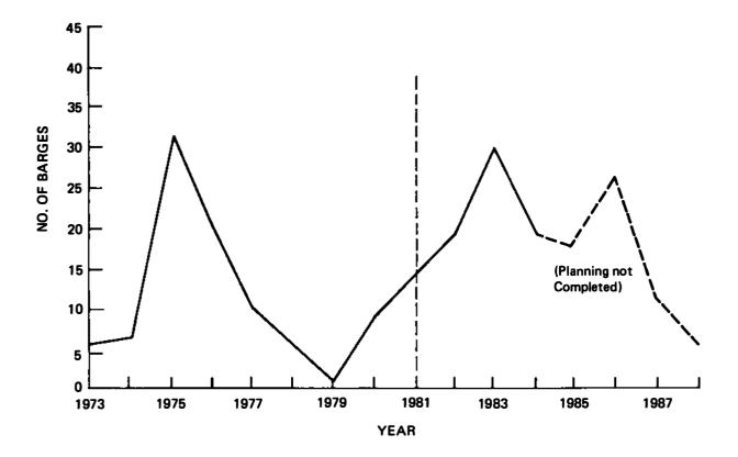
FIGURE 4 1973-1988 trend and projection for North Slope sealift barge requirement expressed in 400' x 100' barge equivalents. Discovery could change barge volume drastically in 1985, and following years.
