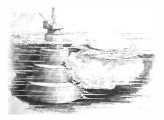
FIGURE 7 Stepped pyramid concept for deep water.
