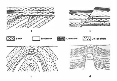
FIGURE 3-1 Different types of oil traps. For simplicity, the reservoir beds are always indicated as sands: (a) stratigraphic trap, (b) structural trap, (c) anticline, (d) salt dome or diapir. (Reprinted from Ross 1982b)
