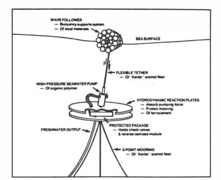
FIGURE 7-2 Pump used in wave energy desalinization device designed by scientists at the University of Delaware. (University of Delaware)
