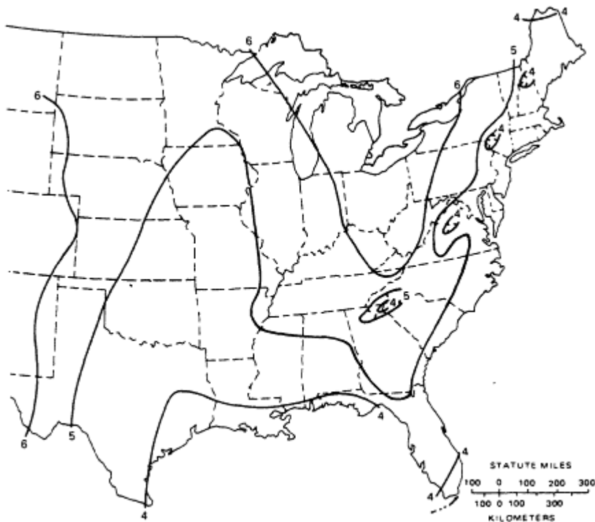
Figure C-2 Ratios of estimated PMP for 10 square miles to estimated 100-year frequency rainfalls (both for 24-hour durations), eastern United States. Source: Riedel and Schreiner (1980).
